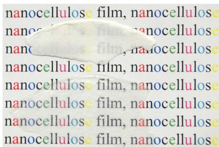
**Figure 4.** Cellulose films obtained from the pulp only treated with a colloidal mill (top, Figure 1C), and additionally treated with the high-pressure homogenizer (bottom, Figure 1D). Hydrogels obtained after sonication of the cellulose suspension did not form films upon drying.
