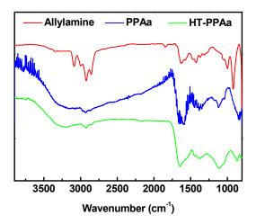
**Figure 1.** Fourier transform infrared spectrum (FTIR) results of allylamine, plasma polymerized polyallylamine film (PPAa), and annealed polyallylamine film (HT-PPAa) film.
