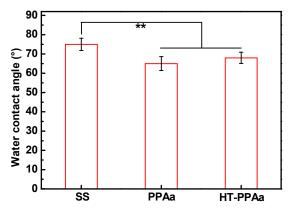
**Figure 3.** The water contact angle of stainless steel (SS), PPAa, and HT-PPAa film. Data are presented as mean  $\pm$  SD (n = 4) and analyzed using one-way ANOVA (\* p < 0.05, \*\* p < 0.01, and \*\*\* p < 0.001).
