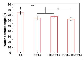
**Figure 9.** The water contact angle of SS, PPAa, and HT-PPAa and BSA-HT-PPAa film. Data are presented as mean  $\pm$  SD (n = 4) and analyzed using one-way ANOVA (\* p < 0.05, \*\* p < 0.01, and \*\*\* p < 0.001).
