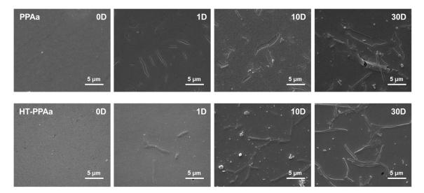
**Figure 6.** The SEM images of PPAa film and HT-PPAa film immersed into the phosphate-buffered saline (PBS) solution for 30 days.
