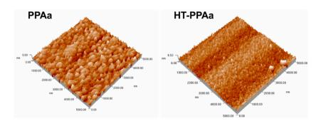
Figure 2. Atomic Force Microscopy (AFM) results of the PPAa and HT-PPAa film surface topography.
