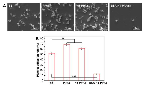
**Figure 10.** (**A**) The platelet adhesion rate of SS, PPAa, HT-PPAa, and BSA-HT-PPAa film. (**B**) Data are presented as mean  $\pm$  SD (n = 4) and analyzed using one-way ANOVA (\* p < 0.05, \*\* p < 0.01, and \*\*\* p < 0.001).
