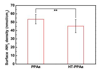
**Figure 5.** Surface -NH<sub>2</sub> density of the PPAa and HT-PPAa samples. Data are presented as mean  $\pm$  SD (*n* = 4) and analyzed using one-way ANOVA (\* *p* < 0.05, \*\* *p* < 0.01, \*\*\* *p* < 0.001).
