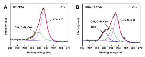
Figure 7. High-resolution survey of (A) HT-PPAa film and (B) BSA-HT-PPAa film on C1s.
