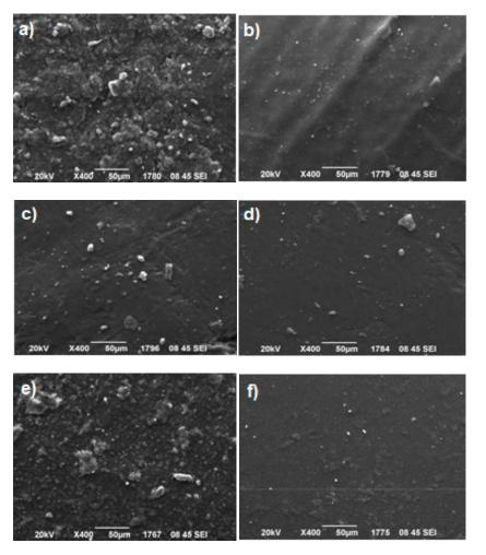
Figure 4. Scanning electron microscopy (SEM) images of a series of experimental dental nanocomposite resins containing (a) Nanomer<sup>®</sup> I.34MN; (b) Montmorillonite-dimethylaminooctadecyl methacrylate (MMT-DMAODM); (c) Montmorillonite-dimethylaminohexadecyl methacrylate (MMT-DMAHDM); (d) S.MMT-DMAHDM; (e) Montmorillonite-cetyltrimethylammonium chloride (MMT-CTAC); (f) S.MMT-CTAC at concentration 50 wt %.
