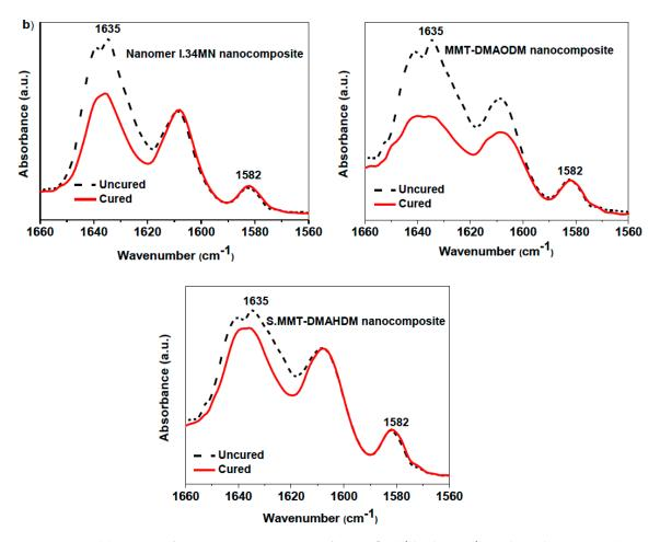
**Figure 5.** (a) Degree of conversion versus time of 2,2-Bis[p-(2'-hydroxy-3'- methacryloxypropoxy) phenylene]propane/triethylene glycol dimethacrylate(Bis-GMA/TEGDMA) matrix and dental nanocomposite resins filled with different OMMT nanoparticles; (b) FTIR spectra with measured peak areas (1635 and 1582 cm<sup>-1</sup>) used to calculate the percent degree of conversion (DC (%)) for uncured and cured nanocomposites.
