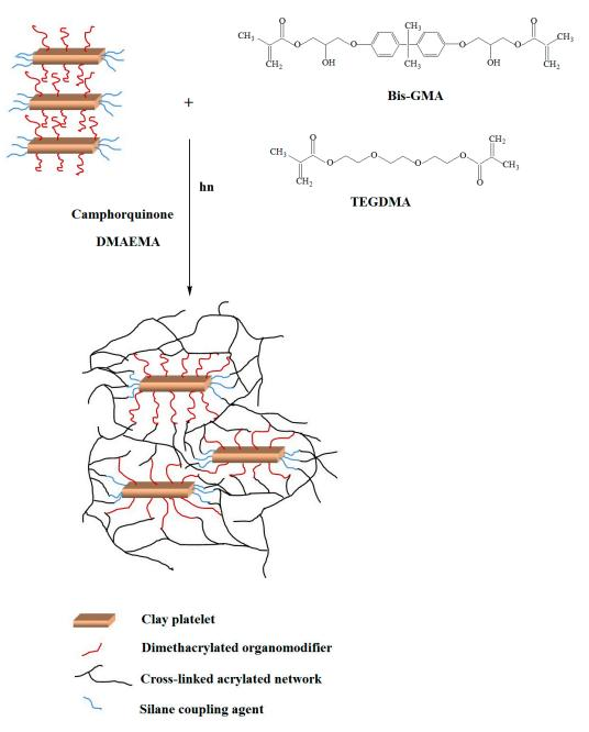
**Figure 3.** Schematic representation of nanocomposite formation indicating the possible chemical interactions between nanoclayorganomodifier and dental resin monomers.
