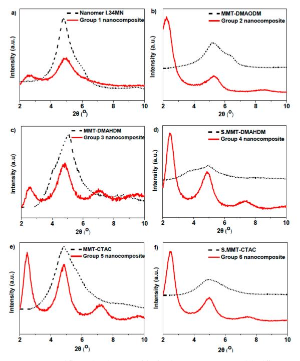
**Figure 2.** X-ray diffraction (XRD) patterns of the dental nanocomposite resins and the different incorporated organo modified montmorillonite (OMMT) nanoclays.
