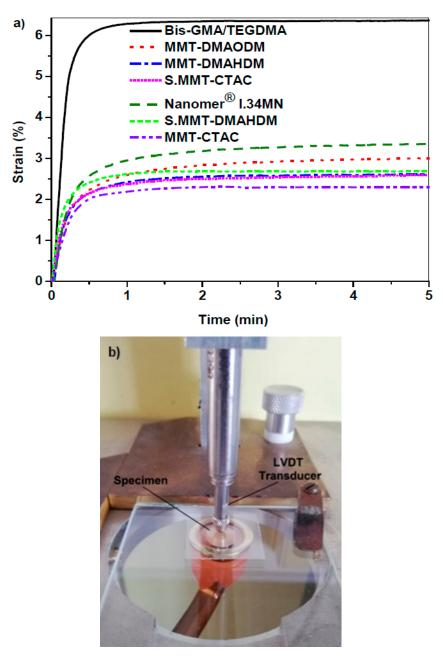
**Figure 7.** (a) Time dependence of polymerization shrinkage strain of Bis-GMA/TEGDMA matrix and dental nanocomposite resins with diverse types of OMMT nanoclays; (b) Apparatus utilized for polymerization shrinkage measurements.
