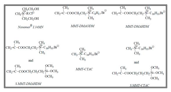
**Figure 1.** Different types of clay organomodifiers used for nanocomposite synthesis (R stands for hydrogenated tallow).
