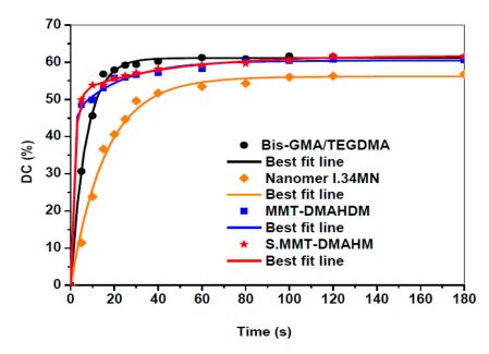
**Figure 6.** Representative DC-time experimental data and the two exponential approximate functions, for pure Bis-GMA/TEGDMA matrix and nanocomposites filled with Nanomer<sup>®</sup> I.34MN, MMT-DMAHDM and S.MMT-DMAHDM. Lines of best fit are drawn through all experimental points of the approximate function.
