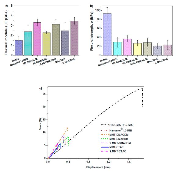
**Figure 8.** (a) Flexural modulus; (b) Flexural resistance; (c) Graphic representation of force against the displacement of flexural properties, for pure Bis-GMA/TEGMA matrix and dental nanocomposite resins filled with different OMMT nanofillers.
