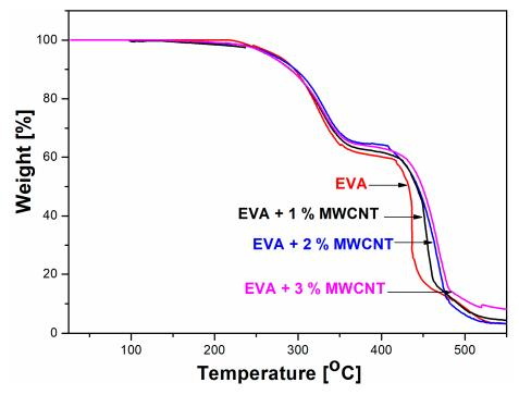
Figure 8. Thermogravimetric analysis (TGA) curves of selected samples.
