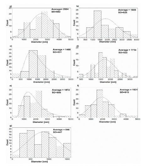
**Figure 3.** Histograms of the prepared samples: (**a**) Pure EVA, (**b**) EVA/0.1 wt % MWCNTs, (**c**) EVA/1.0 wt % MWCNTs, (**d**) EVA/1.5 wt % MWCNTs, (**e**) EVA/2.0 wt % MWCNTs, (**f**) EVA/2.5 wt % MWCNTs, and (**g**) EVA/3.0 wt % MWCNTs.
