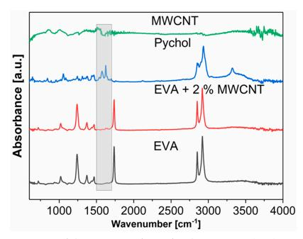
**Figure 5.** Comparison of the Fourier transform infrared spectroscopy (FTIR) spectra of EVA, the compatibilizer cholesteryl 1-pyrenecarboxylate (PyChol), MWCNTs, and EVA/2.0 wt % MWCNTs.
