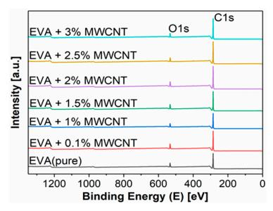
**Figure 6.** X-ray photoelectron spectroscopy (XPS) survey spectra of prepared samples of pure EVA fibers and EVA/MWCNT composites with various wt % of filler.
