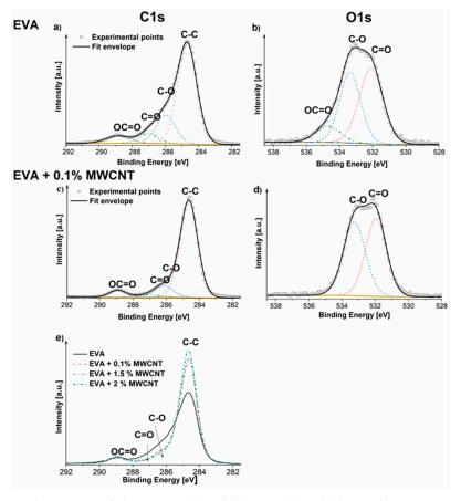
**Figure 7.** C1s and O1s scans of electrospun (**a**) and (**b**) EVA, (**c**), and (**d**) EVA/ 0.1 wt % MWCNTs, and (**e**) C1s comparison of selected samples.
