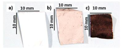
**Figure 1.** Images of selected electrospun samples collected on aluminium foil: (**a**) Pure ethylene vinyl acetate (EVA), (**b**) EVA/1 wt % multiwall carbon nanotubes (MWCNTs), and (**c**) EVA/3 wt % MWCNTs.
