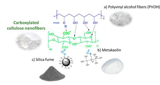
**Figure 4.** Potential interactions between carboxylated CNF and the different components of the C-FCC matrix, such as (**a**) polyvynil alcohol fibers (PVOH); (**b**) metakaolin; and (**c**) silica fume.
