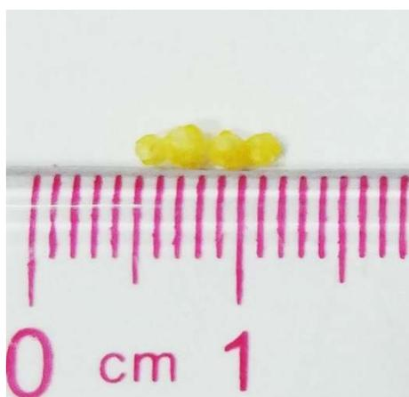
**Figure 9.** A photograph of the PCU coatings after the release of urea in an aqueous solution.
