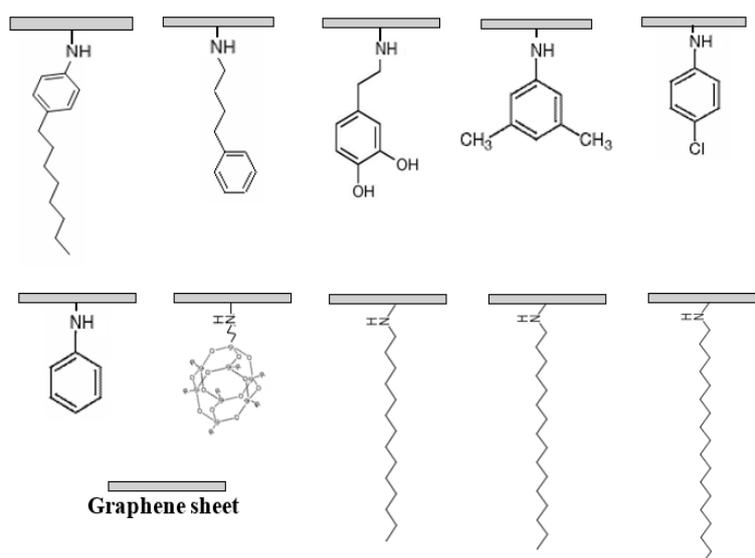
**Figure 1.** Chemical structures of various functionalized-graphene sheets (F-GS).
