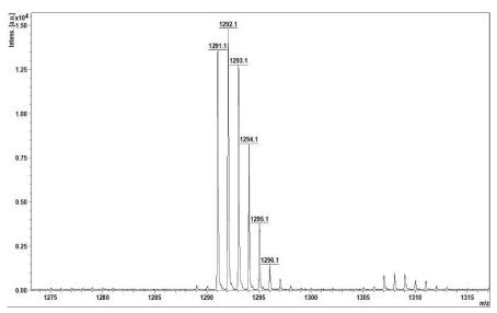
Figure S2. MALDI-TOF mass spectrum of B-POSS.
