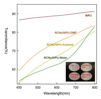
Figure 4. UV-visible spectrums of WPU, RCNs/WPU nanocomposites films.
