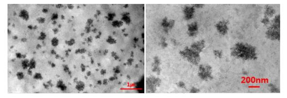
**Figure 1.** TEM micrographs of spherical RCNs prepared by hydrolyzing microcrystalline cellulose (MCC) with a NaOH-based aqueous solution.
