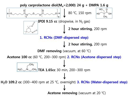
Scheme 1. Regenerated cellulose nanoparticles (RCNs)/waterborne polyurethane (WPU) nanocomposites synthetic process.
