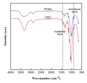
**Figure 2.** FT-IR spectroscopy bands of RCNs prepared by hydrolyzing MCC with a NaOH-based aqueous solution and CNCs by H<sub>2</sub>SO<sub>4</sub> method.
