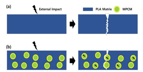
**Figure 13.** Toughening effect according to use of MPCM under external effect: (a) Neat PLA; (b) PLA with MPCM.
