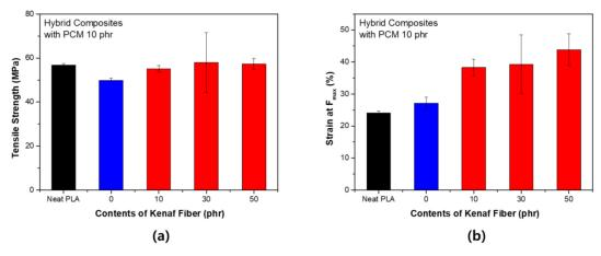
**Figure 4.** Tensile strength of PLA hybrid composites with PCM 10 phr: (a) Maximum stress ( $F_{max}$ ); (b) strain at  $F_{max}$ .
