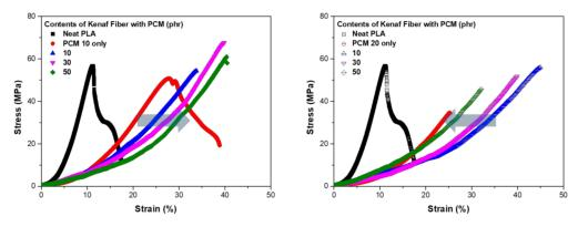
Figure 7. S–S curve from tensile strength test: (a) PCM 10 phr; (b) PCM 20 phr.
