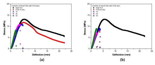
Figure 10. S–S curve of flexural strength test: (a) PCM 10 phr; (b) PCM 20 phr.
