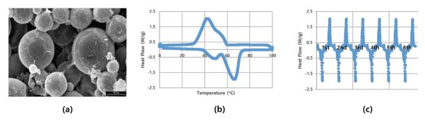
**Figure 1.** Basic characteristics of microencapsulated phase change material (MPCM): (a) SEM image (×2000); (b) endothermic/exothermic reaction (bottom—elevated temperature, above—decreased temperature) with DSC; (c) cycle test with DSC.
