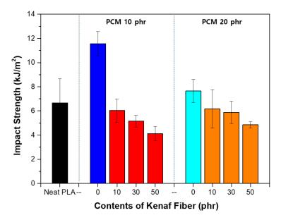
Figure 12. Impact strength of PLA hybrid composites.
