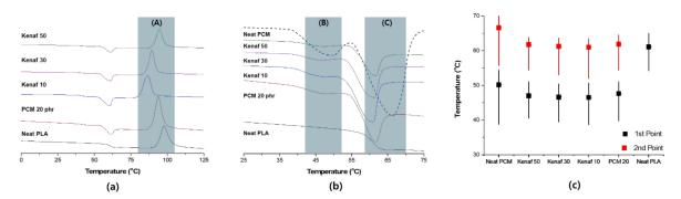
**Figure 3.** Analysis of heat absorption characteristics of PLA hybrid composites with PCM 20 phr: (a) Entire temperature showing the crystallization section (A); (b) expansion of the heat absorption section showing the primary endothermic section (B) and the secondary endothermic section (C); (c) endothermic temperature of each sample.
