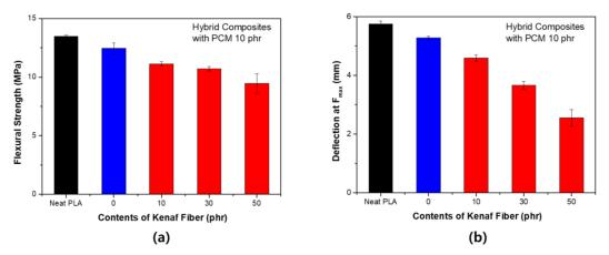
**Figure 8.** Flexural strength of PLA hybrid composites with PCM 10 phr: (a) Maximum stress ( $F_{max}$ ); (b) deflection at  $F_{max}$ .
