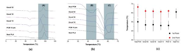
**Figure 2.** Analysis of heat absorption characteristics of PLA hybrid composites with phase change material (PCM) 10 phr: (a) Entire temperature range showing the crystallization section (A); (b) expansion of the heat absorption section showing the primary endothermic section (B) and the secondary endothermic section (C); (c) endothermic temperature of each sample.
