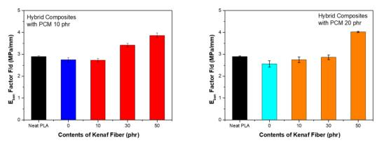
Figure 11. Scale factor of flexural modulus: (a) PCM 10 phr; (b) PCM 20 phr.
