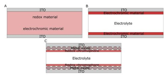
**Figure 3.** Schemes of three different designs of electrochromic devices: (**A**) First type with polymer matrix; (**B**) second type with thin polymer films applied on ITO; (**C**) third type with thin film of metal oxide modified by a redox chromophore.
