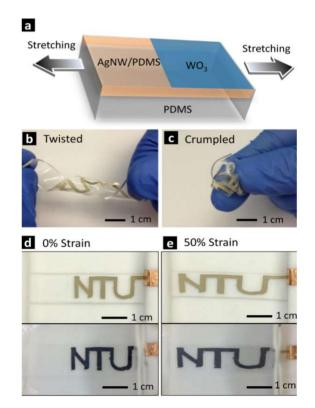
**Figure 4.** Flexible and stretchable electrochromic devices (ECDs) presented by Yan at al. Reprinted with permission from [27]. Copyright 2014, American Chemical Society.
