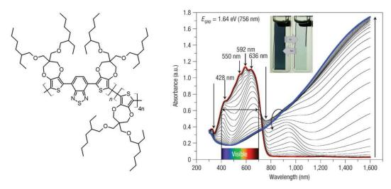
**Figure 5.** Spectroelectrochemistry of a copolymer of alkoxy derivatised poly(3,4-propylenedioxythiophene)-ProDOT and 2,1,3-benzothiadiazole, demonstrating black to transmissive switch upon doping of the polymer layer deposited at ITO electrode. Reprinted with permission and adapted from [30]. Copyright 2008, Springer Nature.
