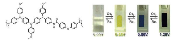
**Figure 6.** Polyamide composed of methoxy functionalised oligotriarylamine and diphenyl ether carboxylic acid units, demonstrating spectacular basic colour multielectrochromism, involving neat transmissive and black states. Reprinted with permission and adapted from [5]. Copyright 2012, The Royal Society of Chemistry.
