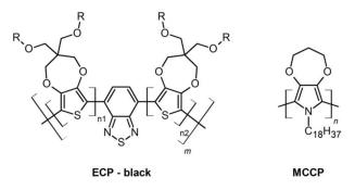
**Scheme 2.** PrODOT/benzothiadiazole copolymer (ECP-Black) used as an active layer and 3,4-propylenedioxypyrrole (MCCP) used as a charge storage layer by Hassab et al. in [41].
