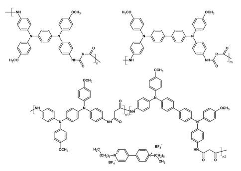
**Scheme 3.** Triphenylamine derivative-based polyamides and a gel electrolyte containing an electrochromic viologen derivative, proposed by Liu et al. in [43].
