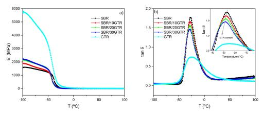
Figure 1. (a) Storage modulus (E'); (b) Damping factor (tanδ) of SBR/GTR compounds.
