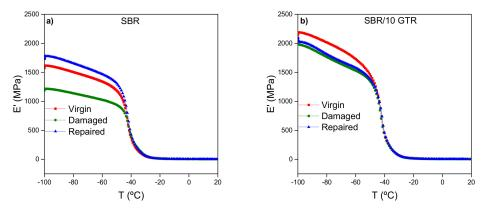
Figure 4. Storage modulus (E') as a function of temperature for: (a) SBR and (b) SBR/10GTR compound.
