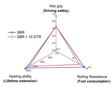
Figure 7. Rolling resistance, wet grip, and healing ability of SBR and SBR/10GTR compounds.
