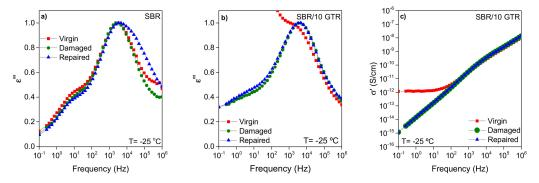
**Figure 5.** Dielectric magnitudes ( $\varepsilon''$  and  $\sigma'$ ) as a function of the frequency at a temperature of  $-25 \degree C$  for the virgin, damaged, and repaired states of: (**a**) SBR; (**b**,**c**) SBR/10GTR compound.
