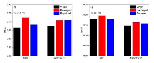
**Figure 6.** Damping factor (tan  $\delta$ ) of SBR and SBR/10GTR compounds under virgin, damaged, and repaired conditions at: (**a**) low temperatures ( $-10 \degree$ C); (**b**) elevated temperatures ( $60 \degree$ C).
