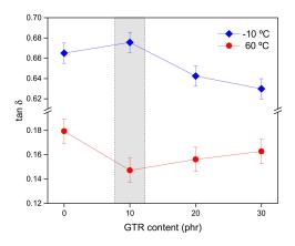
**Figure 2.** Damping factor (tan  $\delta$ ) of SBR/GTR compounds at low (-10 °C) and high (60 °C) temperatures.
