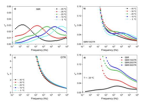
**Figure 3.** Dielectric loss ( $\epsilon''$ ) as a function of frequency in the temperature range from -45 to -5 °C of: (a) SBR compound; (b) SBR/10 GTR compound, and (c) GTR. (d) Dielectric loss ( $\epsilon''$ ) as a function of GTR content at a selected temperature T= -25 °C.
