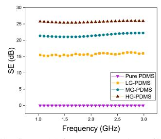
**Figure 4.** EMI shielding effectiveness (SE) of G-PDMS composites with various filler contents (1.1 vol%, 2.3 vol%, 3 vol%, and pure PDMS); the frequency range is 1.0–3.0 GHz.
