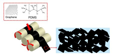
**Figure 1.** Schematic showing the fabrication of a graphene polydimethylsiloxane (G-PDMS) composite using the three-roll milling method. The 2D carbon nano fillers are dispersed by the mechanical shear forces of the rolls.
