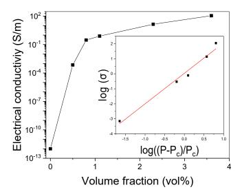
**Figure 3.** Electrical conductivity of the G-PDMS composite as a function of graphene vol% and electrical percolation threshold of a G-PDMS composite. Inset: log-log plot of the conductivity of the composite according to the relation  $((P - P_c)/P_c)$ ; ( $P_c = 0.48$  vol%,  $\beta = 3.9$ ).
