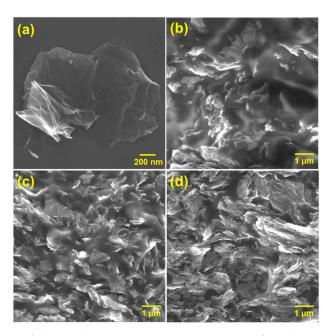
**Figure 2.** SEM image of (**a**) graphene. Cross-section SEM view of (**b**) low graphene (LG)-PDMS, (**c**) middle graphene (MG)-PDMS, and (**d**) high graphene (HG)-PDMS. Graphene is dispersed homogeneously in the polymer.
