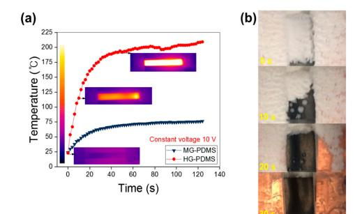
**Figure 5.** Electrical heating performance of G-PDMS according to filler contents at constant voltage (10 V). (a) MG-PDMS film can induce rapid heating performance from room temperature by electrical power. (b) De-icing properties of the HG-PDMS heating unit are superior because of its rapid heating properties.
