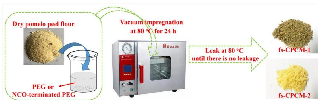
**Scheme 1.** The preparation process for the bio-based form stable composite phase-change materials (fs-CPCMs).
