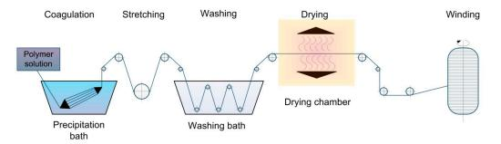
Figure 1. The schematic view of the wet spinning process.
