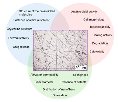
Figure 5. The key detectable parameters of polymer fibers.
