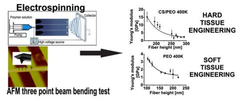
**Figure 8.** The design trend in tissue-engineering scaffolds based on nanomechanical properties of individual electrospun nanofibers. Reprinted with permission from [112].
