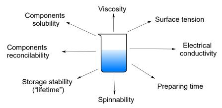
Figure 3. The key detectable parameters of polymeric solutions.
