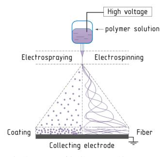
Figure 2. The schematic view of the electrospinning/electrospraying process.
