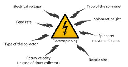
Figure 4. The key technological parameters of the electrospinning process.
