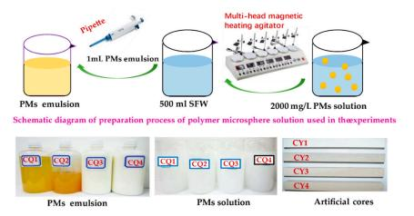
**Figure 2.** Schematic diagram of the preparation process of polymer microsphere solution and photographs of artificial cores and polymer microspheres used in the experiment.
