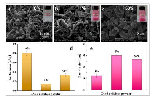
**Figure 6.** (**a**–**c**) SEM images of cellulose powders with varied dye uptake. (**d**) Particle size of cellulose powders with varied dye uptake. (**e**) Surface areas of cellulose powders with varied dye uptake.
