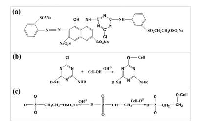
**Figure 4.** (**a**) Chemical structure of B-2BF. (**b**) Nucleophilic substitution reaction between B-type reactive dye and cellulose. (**c**) Nucleophilic addition reaction between B-type reactive dye and cellulose.
