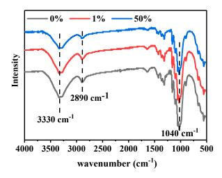
Figure 7. FTIR spectra of 0%, 1%, and 50% owf dyed cellulose powders.
