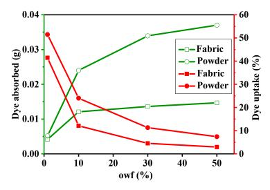
Figure 5. Dye adsorption of powder and fabric with different owfs.
