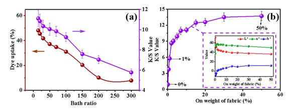
**Figure 2.** (**a**) Influence of bath ratio on K/S value (purple Y-axis pointed by the purple arrow) and dye uptake (brown Y-axis pointed by the brown arrow). (**b**) Relationship between on weight of fabric (owf) and K/S value and the L\*, a\*, and b\* value.
