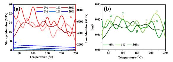
**Figure 10.** (a) Storage (blue Y-axis pointed by blue arrow and blue curves) and loss moduli (red Y-axis pointed by red arrow and red curves) and (b) tan  $\delta$  plots of 0%, 1%, and 50% owf dyed cellulose powders and the  $\alpha$ ,  $\beta$ ,  $\gamma$ , and  $\delta$  transition.
