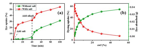
**Figure 3.** (a) Influence of salt on dye uptake. (b) Influence of owf on dye uptake (red Y-axis and red curve) and dye adsorbed (green Y-axis and green curve).
