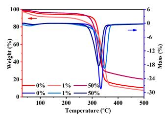
**Figure 9.** Thermal gravity graphs (Weight: red Y-axis pointed by the red arrow; Mass: blue Y-axis pointed by the blue arrow) of cellulose powders with owfs.
