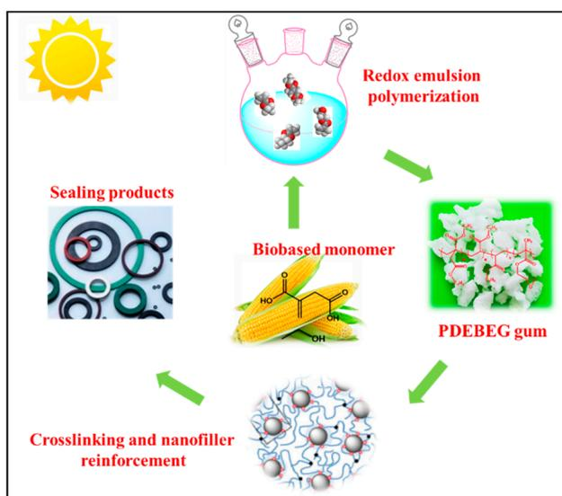
**Figure 1.** Design and preparation route of the novel elastomer with bio-based diethyl itaconate.
