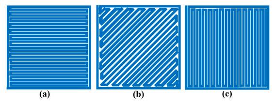
Figure S1 Design of 3D printed hydrogels with different infill angles (a) 0°, (b) 45° and (c) 90°.
