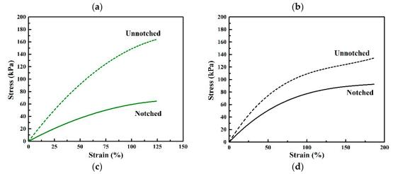
Figure S3 The fitted stress-strain curve of both notched and unnotched sample (**a**) A1S2, (**b**) A1C2, (**c**) A2S2, and (**d**) A2C2.
