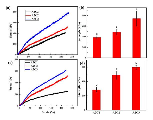
Figure S2, (a) Stress-Stain curve of 3D printed gel with different alginate concentration, (b) strength of 3D printed gels with different agar content (P>0.05), means with different letters are statistically different at P< 0.05, (c) Stress-stain curve of 3D printed gel with different agar concentration, and (d) strength of 3D printed gels with alginate content (P>0.05), means with different letters are statistically different at P<0.05
