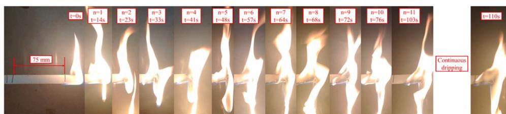
**Figure 11.** The combustion process of PP sample during UL-94 horizontal burning test.
