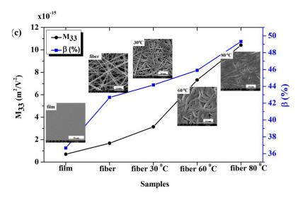
Figure 9. Strain behaviors of film, fibers, and compressed fibers as a function of the (a) electric field and (b) square of the electric field at 1 Hz. (c) The effect of the compression fibers on the electrostrictive coefficients and absolute  $\beta$  fraction.
