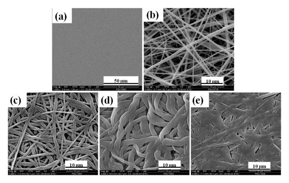
**Figure 3.** SEM images of the P(VDF-HFP) (**a**) film, (**b**) fiber, (**c**) 30 °C compressed fibers, (**d**) 60 °C compressed fibers, and (**e**) 80 °C compressed fibers.
