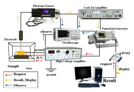
Figure 2. The electrostriction setup.
