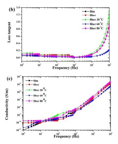
**Figure 7.** Variation of the dielectric constant (**a**), loss tangent (**b**) and AC conductivity (**c**) with frequencies from  $10^0$  to  $10^5$  Hz for the film, fibers, and compressed fiber mats.
