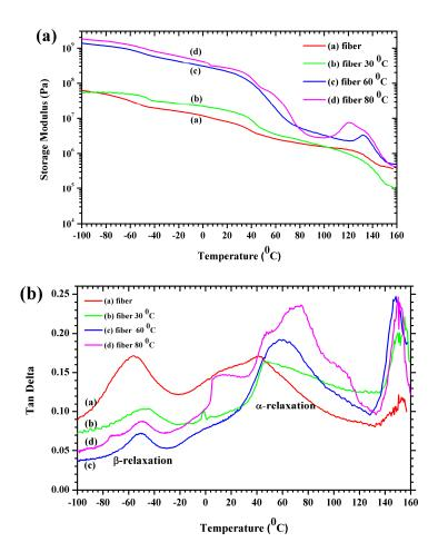
**Figure 6.** The dynamic mechanical analysis curves of P(VDF-HFP) fiber and compressed fiber mats. (a) Storage modulus and (b) tan delta.
