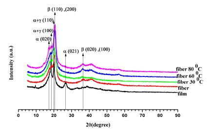
**Figure 4.** X-ray diffractograms for P(VDF-HFP) film, fiber, and fiber mats compressed at 30°, 60°, and 80 °C.
