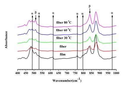
Figure 5. IR spectra of film and fiber P(VDF-HFP) for wavenumbers from 400 to 1000 cm<sup>-1</sup>.
