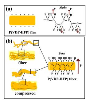
**Figure 8.** Schematic of the proposed  $\beta$ -phase transformation mechanism.
