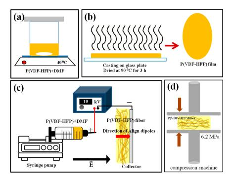
**Figure 1.** Schematic of the synthesis used with all samples. (a) Homogeneous poly(vinylidene fluoride-hexafluoropropylene) (P(VDF-HFP) solution, (b) solution casting, (c) electrospinning, and (d) fibrous film compression.
