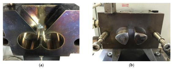
Figure 2. Pictures of measuring mixer (a) mixer bowl with an opening on the top to fill testing material (b) mixing blades on the rear site.
