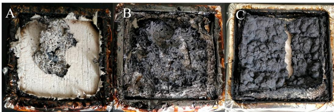
**Figure 4.** Digital images of char residue obtained from cone calorimeter test: (A) TAD0; (B) TAD12; and (C) TAD6EG6.
