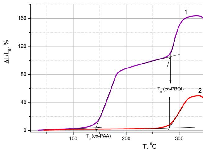
**Figure 7.** Thermomechanical curves of (1) co-PAA and (2) co-PBOI membrane films.
