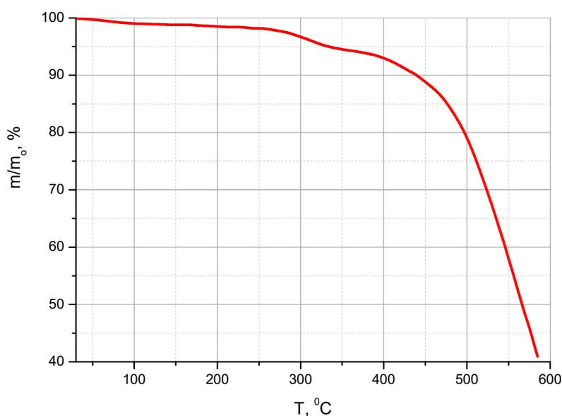
Figure 8. TGA curve of the co-PBOI membrane film.
