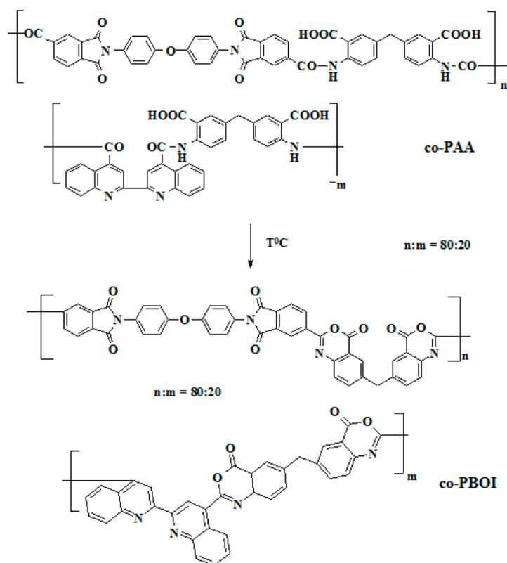
**Figure 1.** Transformation of the co-PAA into the co-PBOI.
