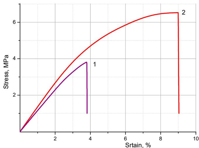
**Figure 6.** Stress–strain curves of (1) co-PAA and (2) co-PBOI membrane films.
