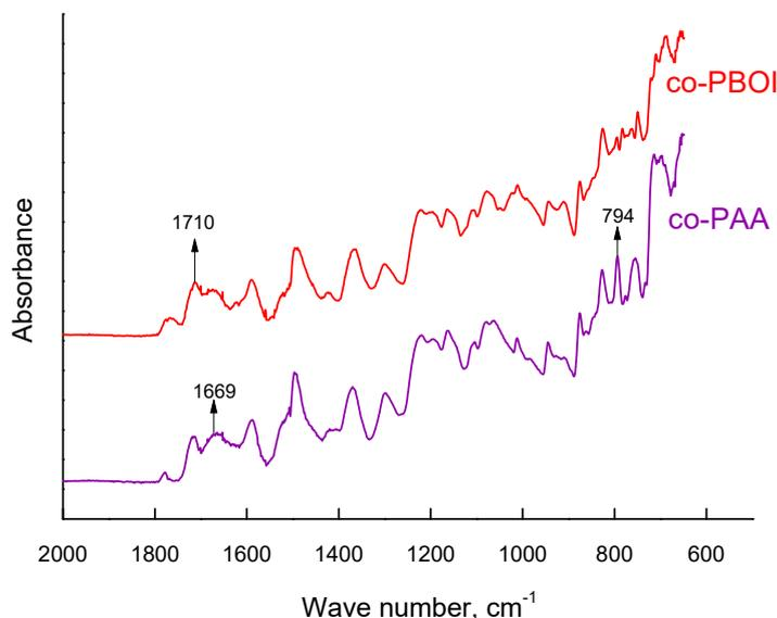
Figure 3. ATR-FTIR spectra of co-PAA and co-PBOI membranes.
