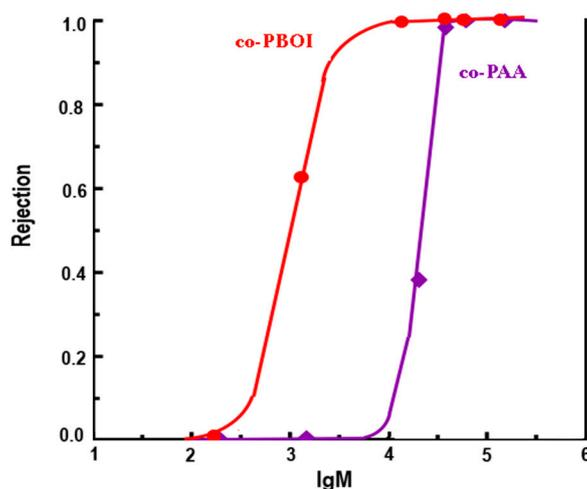
**Figure 9.** Dependence of proteins rejection on their molecular weights in ultrafiltration using co-PAA and co-PBOI membranes.
