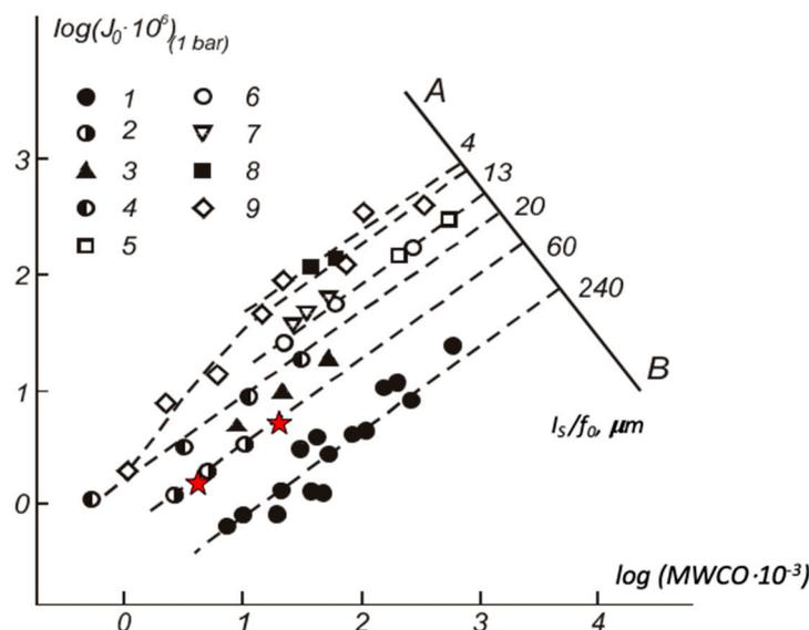
**Figure 10.** Classification diagram of ultrafiltration membranes [37]: 1, Sartorius SM 115–117, and Vladipore UAM, 2, Biopore A2–10, 3, DDS-5,600, –800, 4, Diaflo UM, 5, Biopore A-20-500, 6, Diaflo XM, 7, Dorr-Oliver XP, 8, Diaflo PM, 9, Gelman Omega. Red stars represent the data obtained for co-PAA (right) and co-PBOI (left) membranes.
