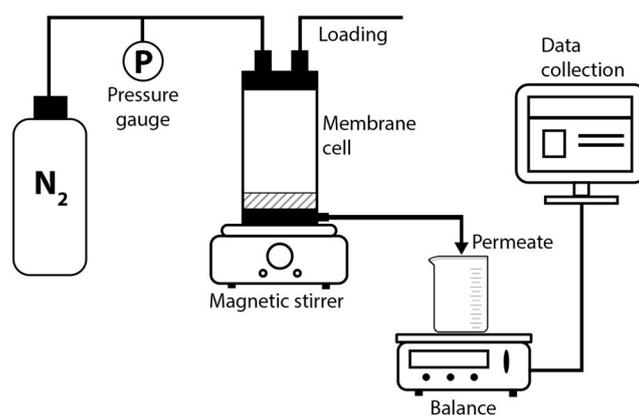
**Figure 2.** Scheme of the laboratory ultrafiltration setup.
