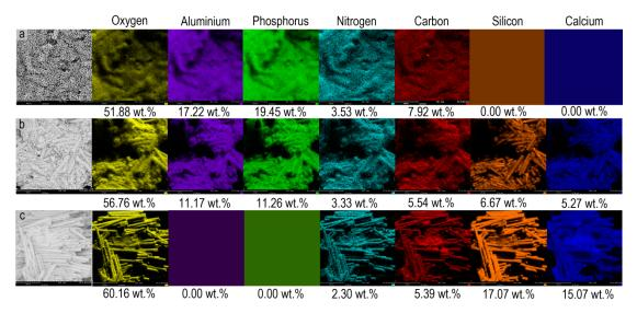
**Figure 4.** EDX scanned photos of surface residue from cone calorimeter tests (**a**) 5%API/7%ADP/GF/PA6; (**b**) 12%ADP/GF/PA6; (**c**) GF/PA6.
