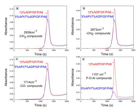
**Figure 6.** Intensity-time curves of typical absorption peak in real-time FTIR spectra of TGA pyrolysis gases of 5%API/7%ADP/GF/PA6 and 12%ADP/GF/PA6. (**a**) –CH<sub>3</sub> compounds; (**b**) –CH<sub>2</sub>– compounds; (**c**) –CO– compounds; (**d**) P–O–Ar compounds.
