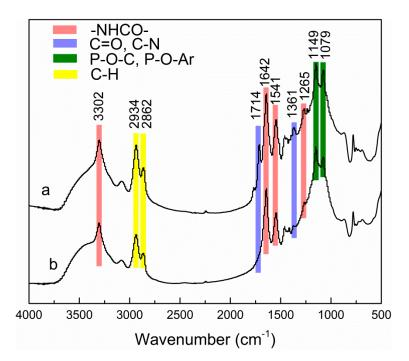
**Figure 5.** FTIR spectra of PA6 composites from cone tests (**a**) 5%API/7%ADP/GF/PA6; (**b**) 12%ADP/GF/PA6.
