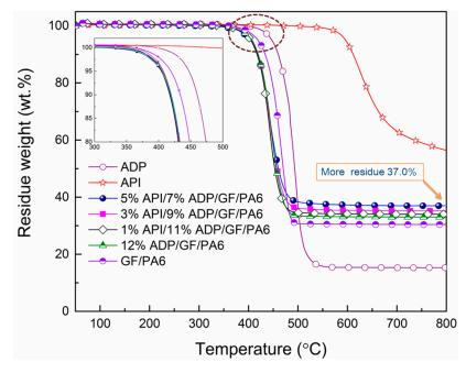
Figure 1. TGA curves for API, ADP and PA6 composites.
