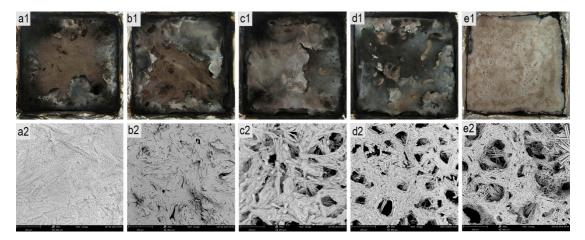
**Figure 3.** Digital photos (**a1–e1**) and SEM photos (**a2–e2**) of residue from cone calorimeter tests (**a1,a2**) 5%API/7%ADP/GF/PA6; (**b1,b2**) 3%API/9%ADP/GF/PA6; (**c1,c2**) 1%API/11%ADP/GF/PA6; (**d1,d2**) 12%ADP/GF/PA6; (**e1,e2**) GF/PA6.
