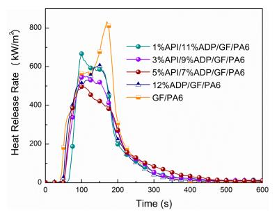
Figure 2. HRR curves of PA6 composites in the cone calorimeter test.
