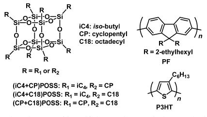
Scheme 1. Chemical structures of the modified POSS and conjugated polymers used in this study.
