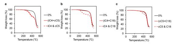
**Figure 2.** TGA profiles of the P3HT hybrids in the absence and presence of: (**a**) 40 wt % (iC4 + CP)POSS and the mixture with 20 wt % iC4-POSS and 20 wt % CP-POSS; (**b**) 40 wt % (iC4 + C18)POSS and the mixture with 20 wt % iC4-POSS and 20 wt % C18-POSS; and (**c**) 40 wt % (CP + C18)POSS and the mixture with 20 wt % CP-POSS and 20 wt % C18-POSS.
