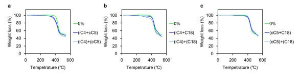
**Figure 1.** TGA profiles of the PF hybrids in the absence and presence of: (a) 40 wt % (iC4 + CP)POSS and the mixture with 20 wt % iC4-POSS and 20 wt % CP-POSS; (b) 40 wt % (iC4 + C18)POSS and the mixture with 20 wt % iC4-POSS and 20 wt % C18-POSS; and (c) 40 wt % (CP + C18)POSS and the mixture with 20 wt % CP-POSS and 20 wt % C18-POSS.
