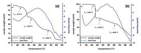
**Figure 7.** TGA curves (weight loss in relation to the initial sample weight) and the corresponding heat flow of (**a**) AZOII and (**b**) AZOIII.
