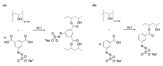
**Figure 8.** Mechanism of coupling reaction of aryl azosulphonates to PVA via polymer analogous esterification reaction: (a) crosslinking of PVA by coupling of AZOII; (b) coupling of monovalent AZOIII to PVA.
