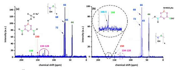
**Figure 9.** <sup>13</sup>C NMR of PAII.5 (comprising 20 wt % of AZOII) before (**a**) and after (**b**) annealing at 100 °C for 60 min.
