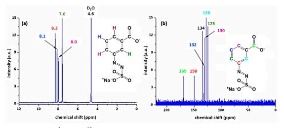
Figure 4. <sup>1</sup>H (a) and <sup>13</sup>C (b) NMR spectra of AZOIII dissolved in deuterated water.
