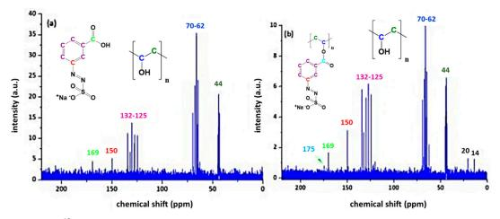
**Figure 10.** <sup>13</sup>C NMR of PAIII.5 (comprising 20 wt % of AZOII) before (**a**) and after (**b**) annealing at 100°C for 60 min.
