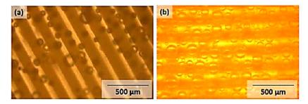
**Figure 15.** Gas bubble formation upon the development of patterned samples (100  $\mu$ m features; dose: 45 Jcm<sup>-2</sup>) in deionised water using phase contrast imaging mode. (a) PAII.5; (b) PAIII.5.
