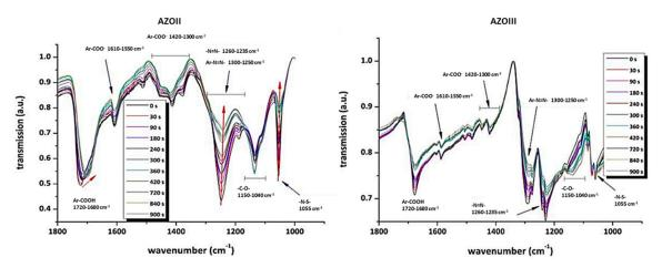
**Figure 5.** FTIR analysis of the AZOII (**a**) and AZOIII (**b**) dye on  $CaF_2$  platelets at different illumination times.
