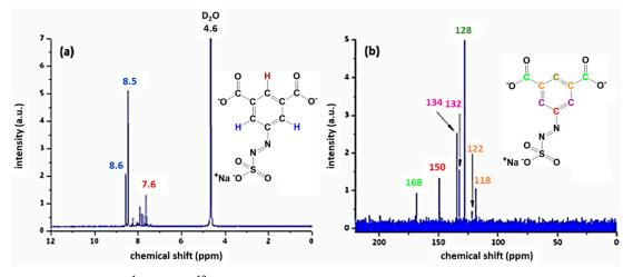
Figure 3. <sup>1</sup>H (a) and <sup>13</sup>C (b) NMR spectra of AZOII dissolved in deuterated water.
