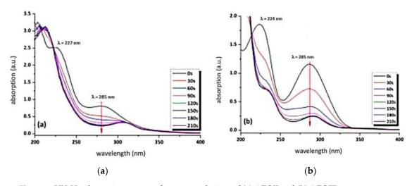
**Figure 6.** UV–Vis absorption spectra of aqueous solutions of (**a**) AZOII and (**b**) AZOIII upon exposure to UV light.
