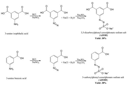
Figure 2. Two-step synthesis of water-soluble aryl azosulphonates.
