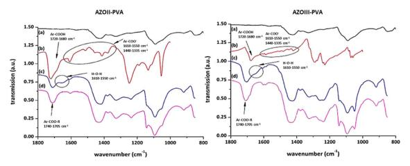
**Figure 11.** FTIR spectra of AZOII-PVA (**left**) and AZOIII-PVA (**right**) polymers; (**a**) neat PVA; (**b**) the respective AZO dye; (**c**) PAII.5/PAIII.5 containing 20 wt % of AZO dye; (**d**) PVA-AZO after 60 min of annealing at 100 °C.
