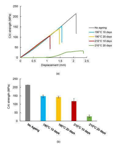
**Figure 8.** CAI test of thermal-aged  $[0/90/\pm 45]_{2s}$  quasi-isotropic laminates. (a) Averaged CAI stress–displacement curves. (b) Average CAI results and standard deviation.
