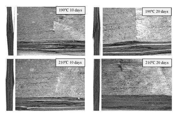
**Figure 9.** CAI damage profiles during the CAI test of  $[0/90/\pm 45]_{2s}$  quasi-isotropic laminates aged at 190 °C and 210 °C for 10 and 20 days. An impact load of 20 J was applied on the front face.
