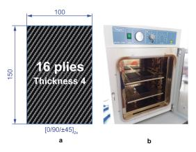
**Figure 1.** (a) Standard impact specimens according to ASTM D7136 recommendations. (b) Programmable oven used for the thermal ageing treatments.
