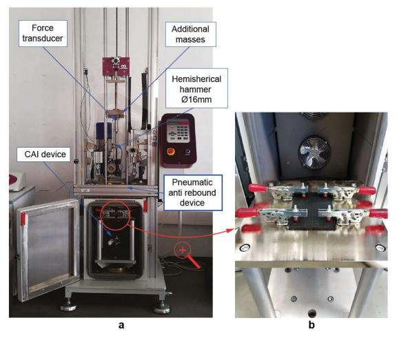
Figure 2. Experimental setup for drop-weight impact test. (a) Drop-weight column device.(b) Compression after impact (CAI) support fixture according to ASTM D7136 standard.
