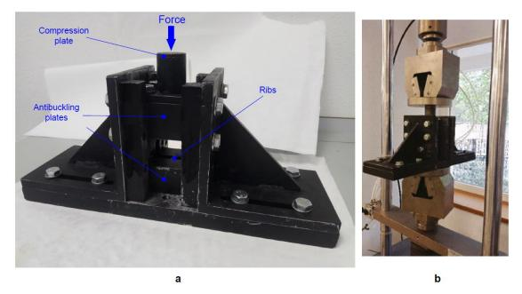
**Figure 5.** (a) Description of the non-standard adjustable CAI device proposed in this study. (b) Experimental setup for CAI testing.
