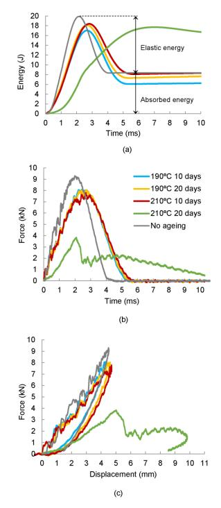
**Figure 6.** (a) Average energy and (b) force histories and (c) force–displacement curves of non-aged  $[0/90/\pm45]_{2s}$  quasi-isotropic composite laminates with different ageing processes.
