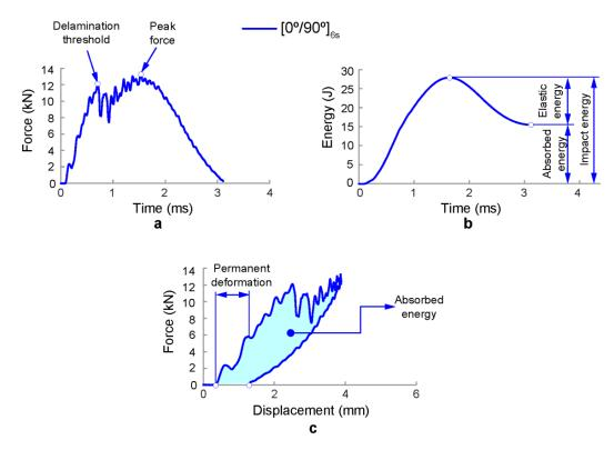
**Figure 3.** Impact damage response histories of typical composite laminates under drop-weight impact test: (**a**) force–time history, (**b**) energy–time history, and (**c**) force–displacement history [3].
