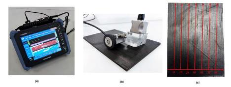
**Figure 4.** Experimental setup of phased array ultrasonic testing. (a) Olympus Omniscan SX. (b) Phased-array transducer of 64 elements at 5 MHz with coupled encoder. (c) Details of the raster scan scheme for the composite laminates.
