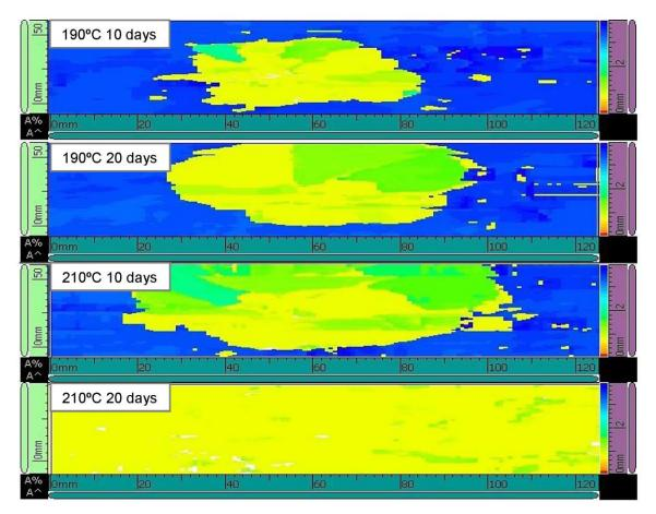
**Figure 7.** Ultrasonic C-scanning images of the damaged area of  $[0/90/\pm 45]_{2s}$  quasi-isotropic composite laminates aged at different temperatures and periods of time. The effect of ageing on the impact damage response. (E<sub>impact</sub> = 20 J).
