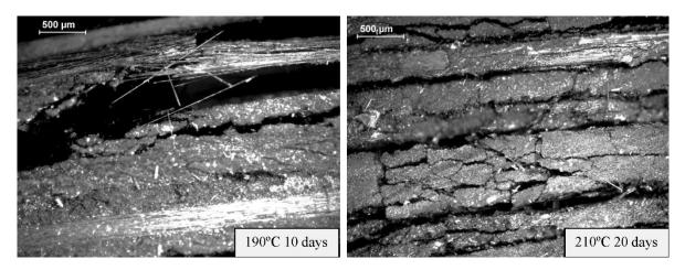
**Figure 10.** Details of the CAI damage profiles during the CAI test of  $[0/90/\pm 45]_{2s}$  quasi-isotropic laminates aged at 190 °C for 10 days and 210 °C for 20 days.
