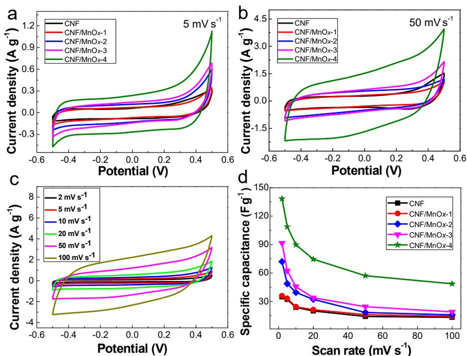
**Figure 5.** Cyclic voltammetry (CV) curves of the CNF/MnO<sub>x</sub> electrodes at a scan rate of (a) 5 mV s<sup>-1</sup> and (b) 50 mV s<sup>-1</sup>. (c) Changes of CV curves of CNF/MnO<sub>x</sub>-4 at scan rates from 2 to 100 mV s<sup>-1</sup>. (d) Specific capacitance vs. scan rate.
