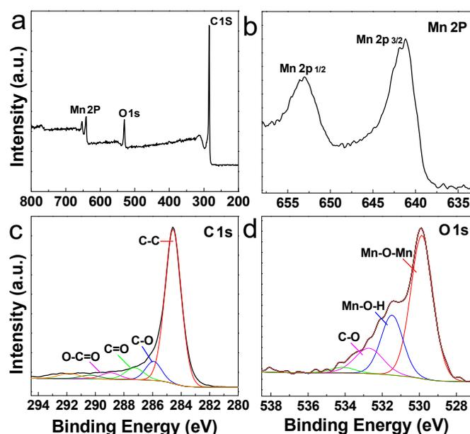
**Figure 3.** (a) X-ray photoelectron spectroscopy (XPS) survey spectrum of CNF/MnO<sub>x</sub>-4. (b–d) XPS high-resolution spectra of Mn 2p, C 1s, and O 1s.
