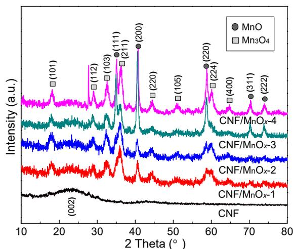
**Figure 4.** X-ray diffraction (XRD) patterns of CNF and CNF/MnO<sub>x</sub> composite aerogels.
