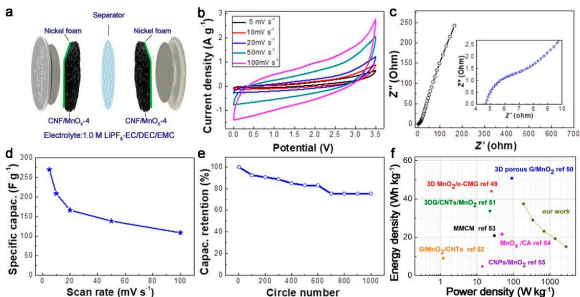
**Figure 7.** Electrochemical measurement of the CNF/MnO<sub>x</sub>-4 based symmetric supercapacitor: (a) Schematic illustration of the CNF/MnO<sub>x</sub>-4-based symmetric supercapacitor; (b) CV curves obtained at different scan rates; (c) Nyquist plots; (d) Specific capacitance vs. scan rate; (e) Cyclic stability at a charge–discharge current density of 2 A g<sup>−1</sup> for 1000 cycles; (f) Ragone plot.
