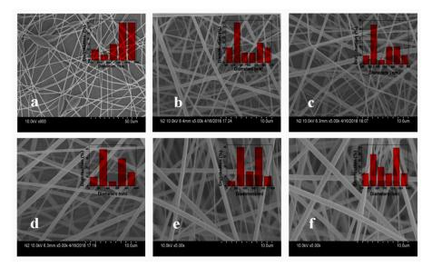
**Figure 2.** SEM micrographs and diameter distributions of the sc-PLA/PMMA nanofibers with *sc*-PLA contents of (**a**) 0 wt %, (**b**) 5 wt %, (**c**) 10 wt %, (**d**) 15 wt %, (**e**) 20 wt % and (**f**) 25 wt %.
