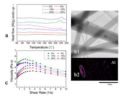
**Figure 3.** Analysis of the fabrication of *sc*-PLA in PMMA. (**a**) DSC melting curves for the different samples with various *sc*-PLA contents. (**b1**) TEM images for *sc*-PLA/PMMA nanofibers with 20 wt % *sc*-PLA contents. (**b2**) EDS mapping of aluminum. (**c**) Change of viscosity with shear rate for various *sc*-PLA contents.
