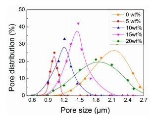
Figure 6. Pore distribution of sc-PLA/PMMA nanofiber filter with different sc-PLA contents.
