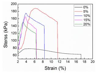
Figure 4. Stress-strain curves of sc-PLA/PMMA nanofiber filter with different contents of sc-PLA.
