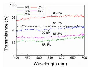
Figure 5. Transmittance of *sc*-PLA/PMMA nanofiber filter with different *sc*-PLA contents.
