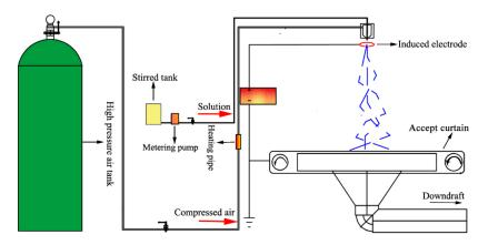
**Figure 1.** Schematic of the preparation of transparent air filter material by electrostatic induction-assisted solution blowing.
