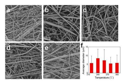
**Figure 1** SEM graphs of the PP fiber prepared by meltblown under different melt temperatures. 220°C (a), 240°C (b), 260°C (c), 280°C (d), 300°C (e). And the fiber diameter analysis of these fabrics (f).
