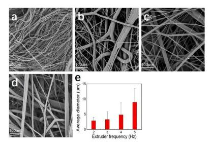
**Figure 3** SEM graphs of the PP fiber prepared by meltblown under different extruder screw rotating speeds. 2 Hz (120 rpm) (a), 3Hz (180 rpm) (b), 4 Hz (240 rpm) (c), 5 Hz (300 rpm) (d). And the fiber diameter analysis of these fabrics (e).
