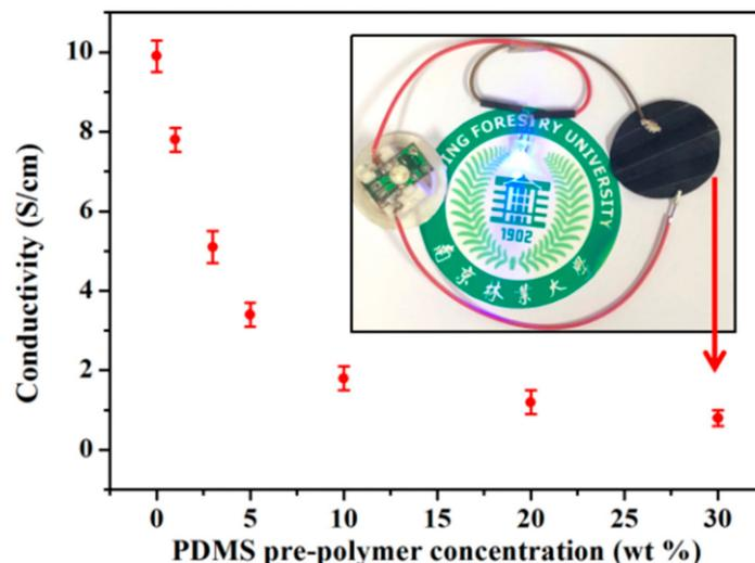
**Figure 3.** Conductivity of PDMS/CNF/CNT depending on the PDMS pre-polymer concentration during the immersion process, and a digital image which shows that the folded PDMS-30/CNF/CNT was used as a wire to let a blue LED glow well (inserted picture).
