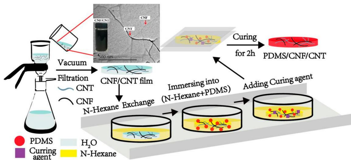
**Figure 1.** Preparation route of Polydimethylsiloxane/cellulose nanofiber/carbon nanotube (PDMS/CNF/CNT) nanocomposite and the TEM image of CNF/CNT mixture suspension (the inserted digital image of CNF/CNT dispersion exhibited uniform appearance even after two months).
