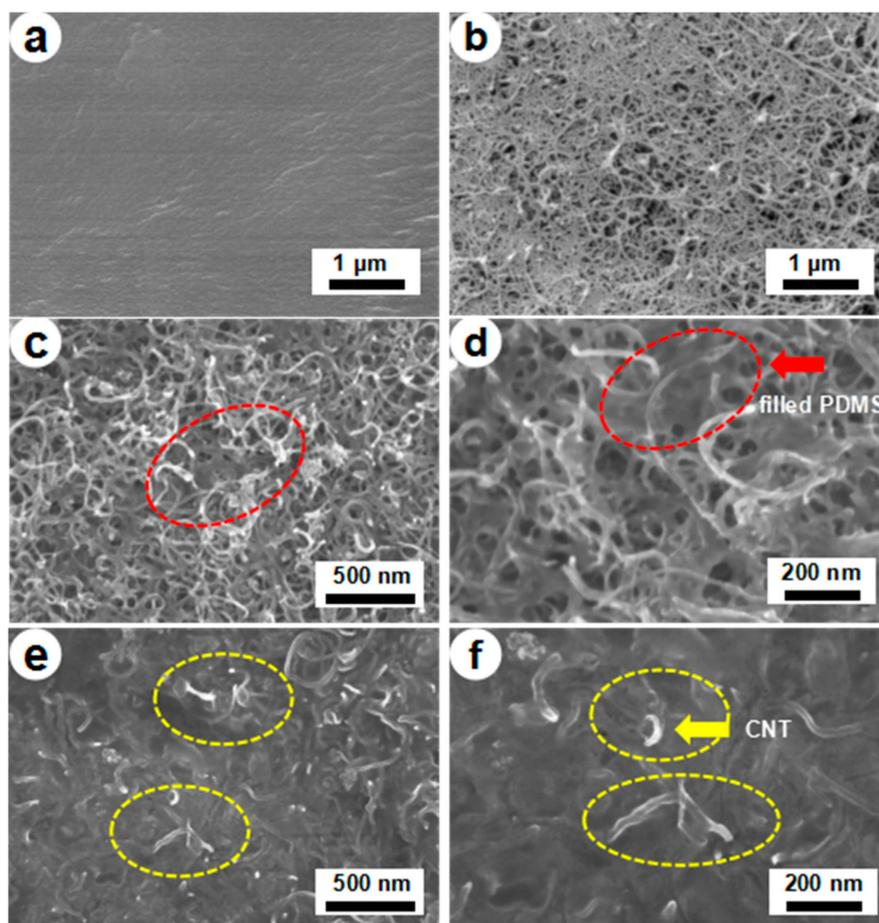
**Figure 2.** Field emission scanning electron microscope (FE-SEM) images of Pure PDMS (a) CNF/CNT (b) PDMS-1/CNF/CNT composite film (c)  $\times 50,000$  (d)  $\times 100,000$  and PDMS-30/CNF/CNT composite film (e)  $\times 50,000$  and (f)  $\times 100,000$ .
