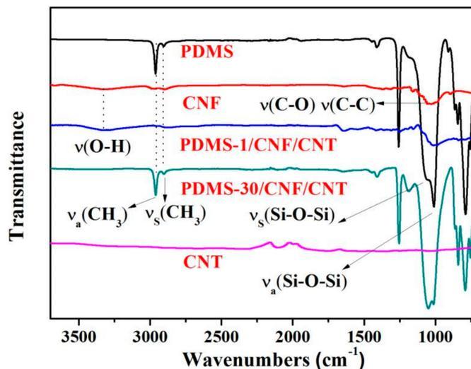
**Figure 5.** FTIR spectra of PDMS, CNF, CNT, and PDMS/CNF/CNT nanocomposite samples.
