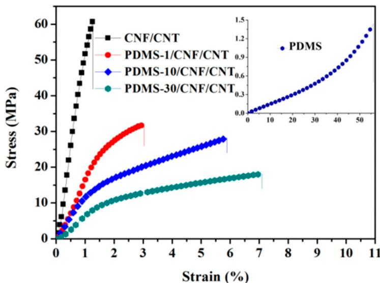
**Figure 6.** Tensile stress-strain curves of the CNF/CNT and PDMS/CNF/CNT composite film in different PDMS content.
