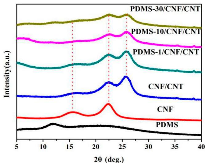
**Figure 4.** X-ray diffraction profiles of PDMS, CNF, CNF/CNT, and PDMS/CNF/CNT nanocomposite film samples.
