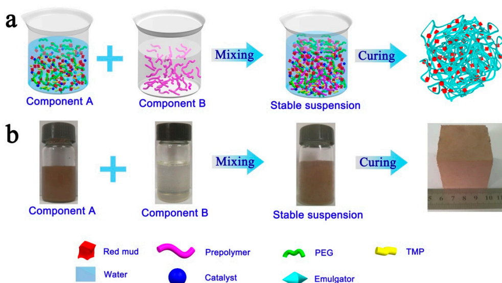
Figure 1. (a) Schematic illustration of the fabrication process of polyurethane/red mud composite (PRC). (b) Digital photographs of component A, component B, stable suspension, and cured PRC.
