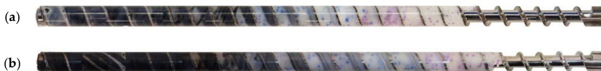
**Figure 4.** Top views of the frozen-screw pulls: (a) General purpose, square-pitched screw; (b) Barrier screw with melt channel, barrier flight, and mixing element.
