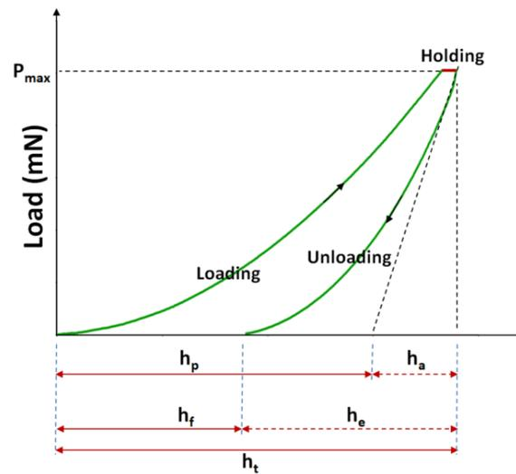
Figure 9. Representative plot of load versus displacement.
