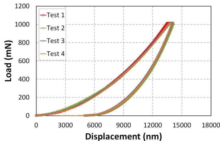
Figure 10. Indentation profile for epoxy matrix, 2.5 wt %NGP.
