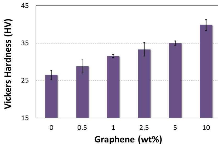
Figure 16. Effect of graphene additives on NGP/epoxy hardness.
