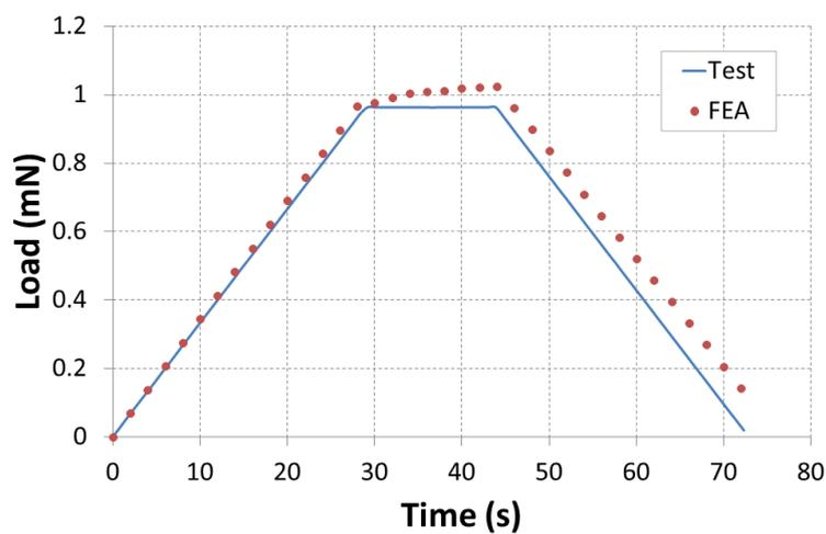
Figure 19. Correlation between the experimental and numerical load.
