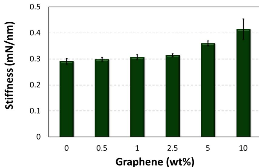
Figure 15. Effect of graphene additives on stiffness.
