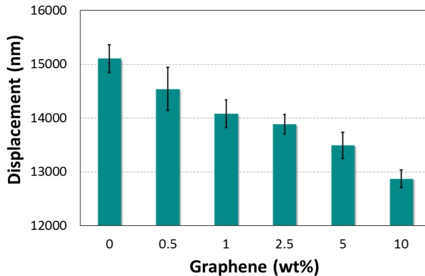
Figure 14. Effect of graphene additives on maximum displacement.
