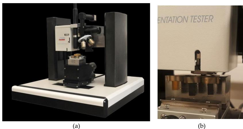
**Figure 5.** Image of (a) the indentation machine and (b) specimens under test.
