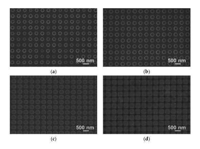
**Figure 3.** The SEM images of Ag nanolens array substrate with (**a**) SiO<sub>2</sub> 50, Ag 100 nm, (**b**) SiO<sub>2</sub> 100, Ag 100 nm, (**c**) SiO<sub>2</sub> 150, Ag 100 nm, and (**d**) SiO<sub>2</sub> 200, Ag 100 nm.
