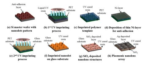
**Figure 1.** A schematic diagram of the plasmonic nanolens array fabrication using the nanoimprinting method.
