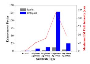
**Figure 7.** The effect of the SiO<sub>2</sub> layer thickness on the fluorescence enhancement factor and maximum electric field intensity at 1  $\mu$ g/mL and 100 ng/mL SA-Cy5 concentrations; the control signal was obtained from bare glass (reference).
