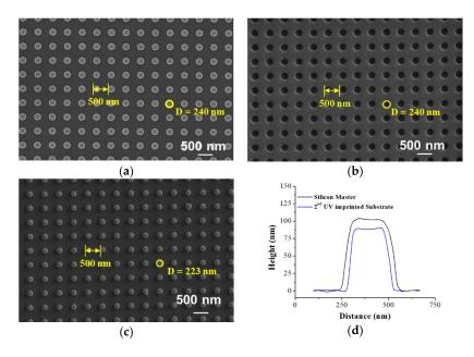
**Figure 2.** The top-view scanning electron microscope (SEM) images of (**a**) silicon master, (**b**) polymer master, (**c**) replicated nanopillar pattern, and (**d**) the comparison of the cross-sectional surface profiles of the silicon master and replicated nanopillar structures on a glass substrate obtained via atomic force microscope (AFM) measured results.
