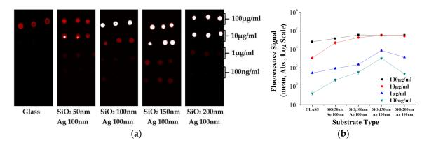
**Figure 5.** The comparison of measured fluorescence (**a**) microarray images and (**b**) intensity values at each streptavidin-Cy5 (SA-Cy5) concentration on the plasmonic nanolens array metal enhanced fluorescence (PNA-MEF) substrate and bare glass substrate (reference).
