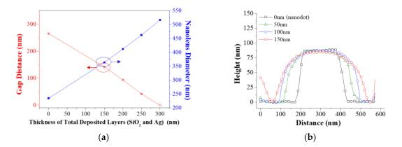
**Figure 4.** (a) The plot of the measured lens-to-lens spacing (left axis, red squares) and diameter (right axis, blue squares), and (b) measured AFM profiles of the nanolens structures as a function of the SiO<sub>2</sub> layer thickness.
