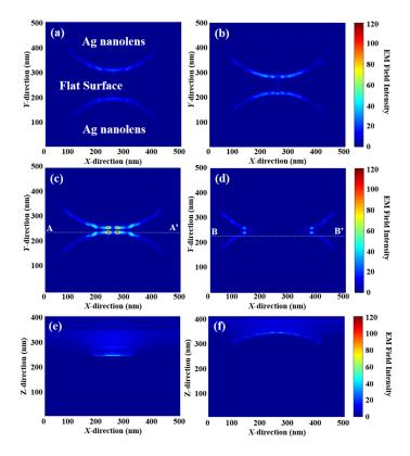
**Figure 6.** The RCWA simulation results of the EM field intensity distribution of PNA-MEF substrate with (**a**) 50, (**b**) 100, (**c**,**e**) 150, and (**d**,**f**) 200 nm SiO<sub>2</sub> and 100 nm Ag layers; (**a**–**d**) *x*-*y* plane distribution at the PNA base plane and (**e**,**f**) the *x*-*z* plane distribution where the maximum EM field intensity was located; (**e**) the A-A' line cross-section and (**f**) the B-B' line cross-section.
