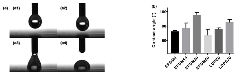
**Figure 2.** Hydrophobic properties of the fluorinated EPDM and LDPE. (a) Hydrophobicity measurement; (b) contact angle.
