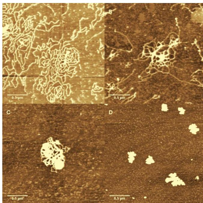
**Figure 8.** The AFM images of DNA condensation induced by  $\text{Co}^{3+}$ . The concentration of  $\text{Co}^{3+}$  is 0.01 mM (A); 0.06 mM (B); 0.15 mM (C); and 0.2 mM (D).
