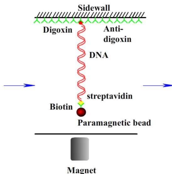
**Figure 1.** A schematic diagram of magnetic tweezers.
