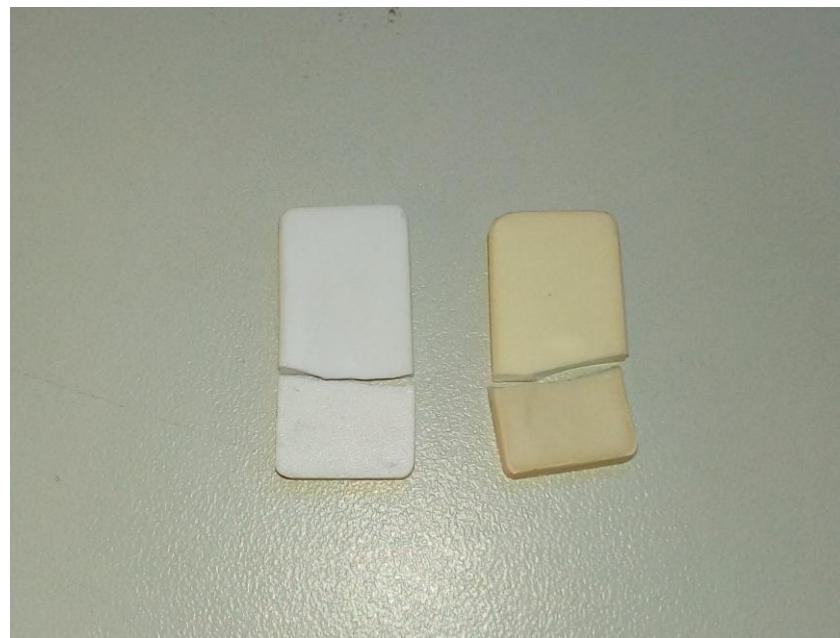
**Figure S8.** Pre-and post-aged samples of cured materials for impact tests.
