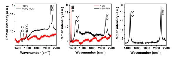
**Figure 3.** Raman spectra measured on: (a) pristine HOPG and HOPG after diacetylene deposition and UV irradiation for 20 min; (b) pristine h-BN and h-BN after diacetylene deposition and UV irradiation for 10 s; and (c) the diacetylene powder after UV irradiation for 10 s.
