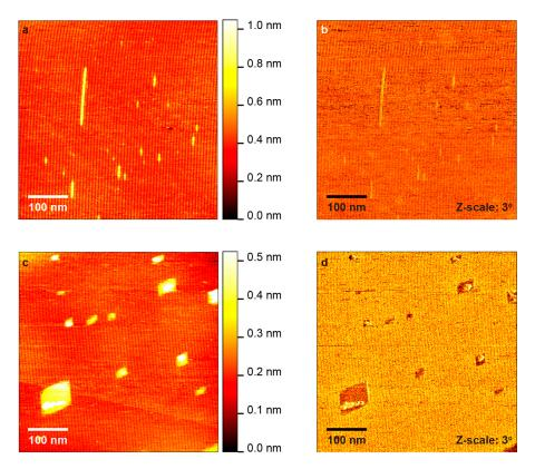
**Figure 2.** AFM topography (**a**); and phase shift (**b**) of diacetylene on hexagonal-Boron Nitride (h-BN) after 5 s of UV irradiation; and the same sample after additional 5 s of irradiation (10 s in total) (**c**) topography; (**d**) phase shift.
