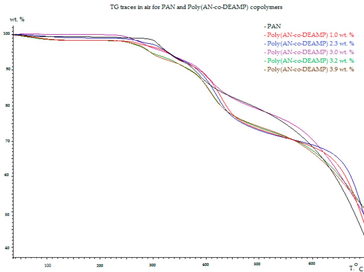
Figure S1. TG traces obtained under air for PAN and the copolymers poly(AN-co-DEAMP) containing different amounts of phosphorus.
