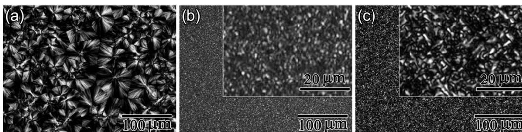
**Figure 8.** POM micrographs for fully crystallized samples of (a) PLA-U; (b) PLA-T0; and (c) PLA-T35. The insets in panels b–c show high-magnification images.
