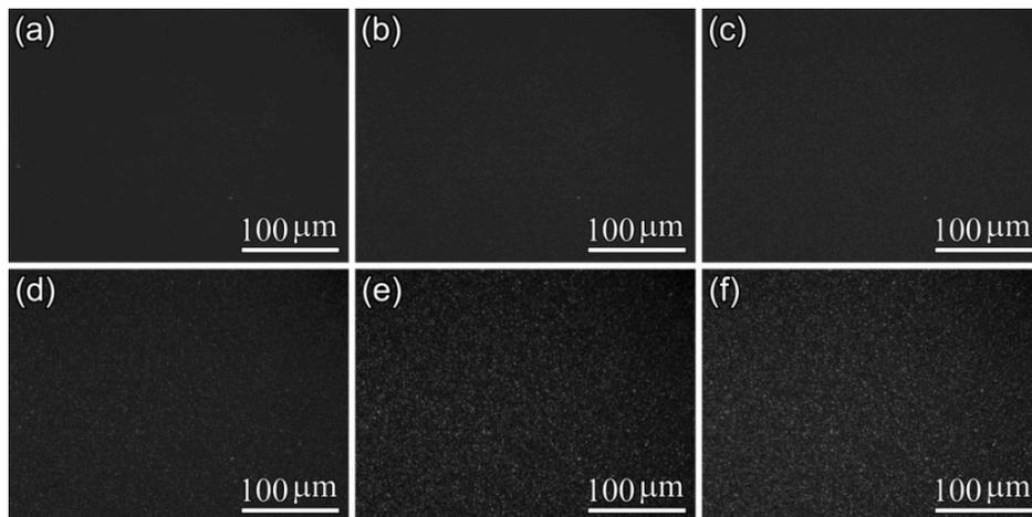
**Figure 6.** POM micrographs of PLA-T0 film during isothermal crystallization at 110 °C: (a) 0 min; (b) 6 min; (c) 9 min; (d) 13 min; (e) 20 min; and (f) 30 min.
