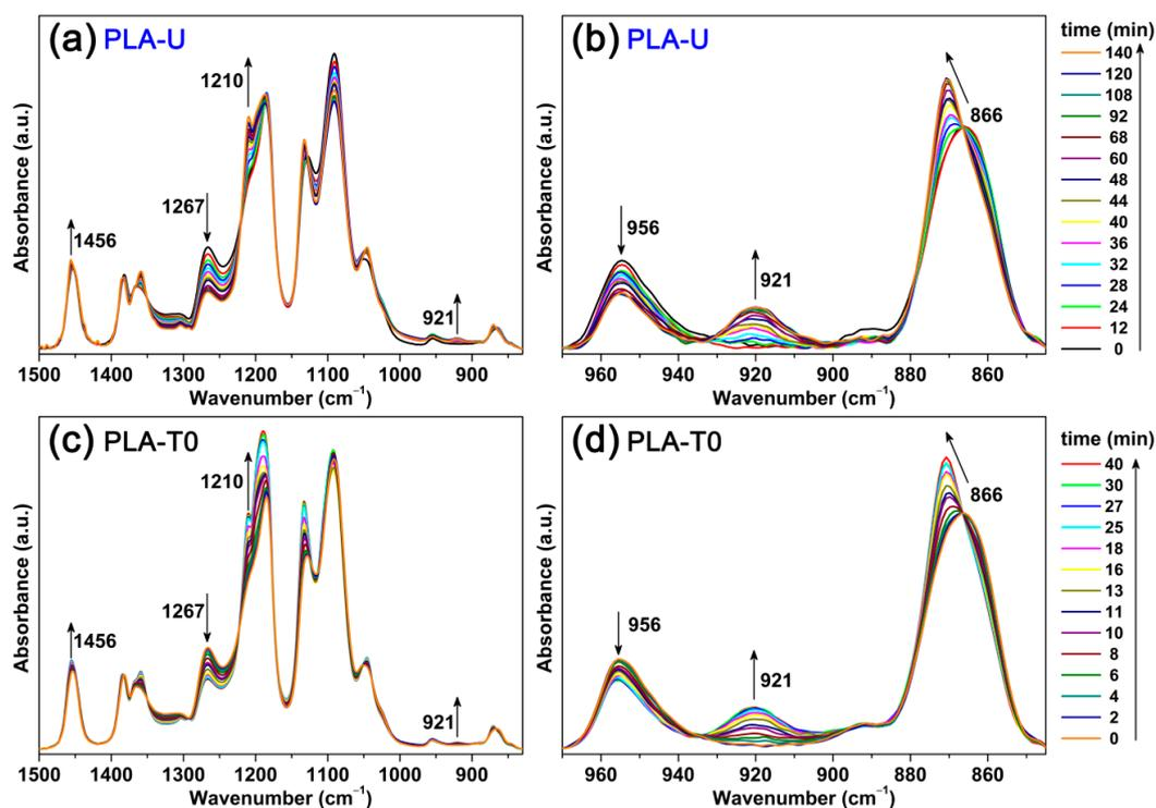
**Figure 3.** Time-resolved FTIR spectra in the 1500–830 cm<sup>-1</sup> (a,c) and 970–850 cm<sup>-1</sup> (b,d) ranges for PLA-U (a,b) and PLA-T0 (c,d) during the isothermal crystallization at 110 °C.
