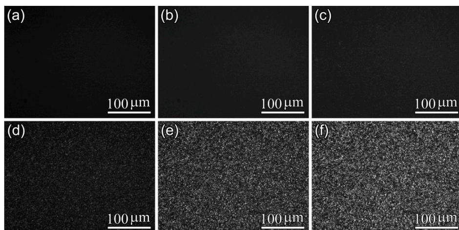
**Figure 7.** POM micrographs of PLA-T35 film during isothermal crystallization at 110 °C: (a) 0 min; (b) 6 min; (c) 9 min; (d) 13 min; (e) 20 min; and (f) 30 min.
