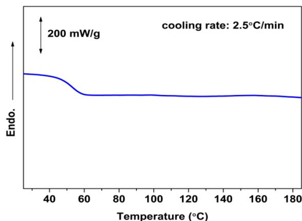
**Figure 1.** DSC cooling curves for untreated PLA sample (PLA-U) at a cooling rate of 2.5 °C/min from the melt.
