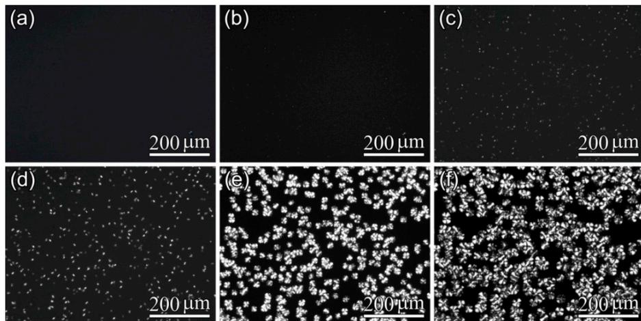
**Figure 5.** POM micrographs of PLA-U film during isothermal crystallization at 110 °C: (a) 0 min; (b) 20 min; (c) 30 min; (d) 40 min; (e) 90 min; and (f) 120 min.
