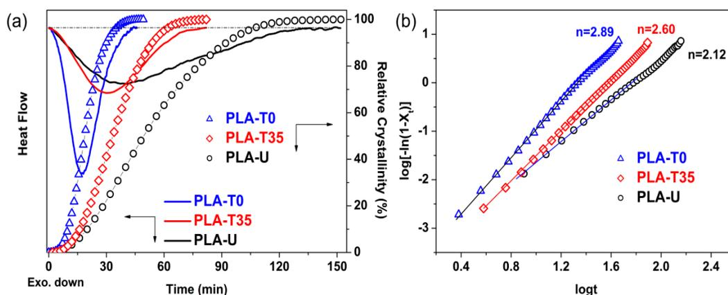
**Figure 2.** (a) DSC traces and variation of relative crystallinity with crystallization time for PLA-U, PLA-T35, and PLA-T0 at 110 °C and (b) the corresponding Avrami plots.
