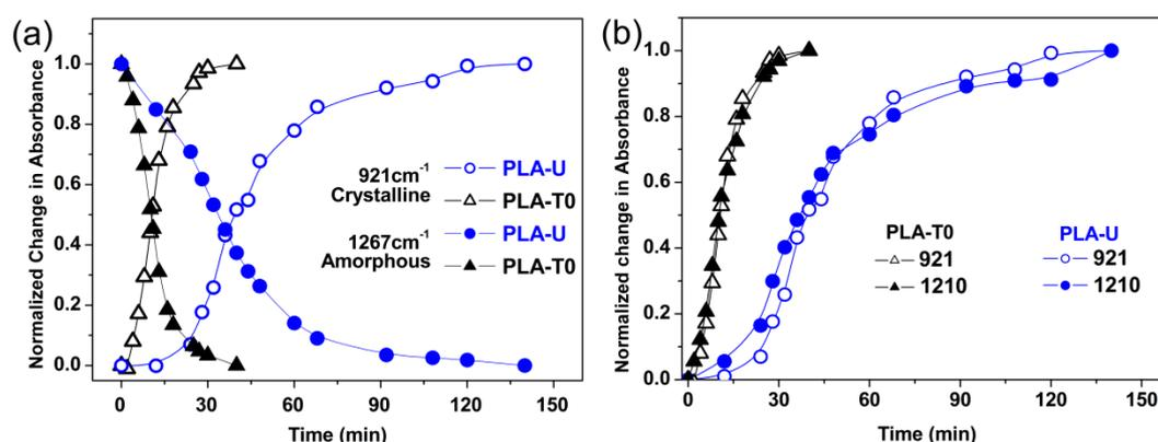
**Figure 4.** (a) Normalized changes in absorbance for crystalline ( $921\text{ cm}^{-1}$ ) and amorphous ( $1267\text{ cm}^{-1}$ ) bands for PLA-U and PLA-T0; (b) Normalized changes in absorbance for crystalline ( $921$  and  $1210\text{ cm}^{-1}$ ) bands for PLA-U and PLA-T0.
