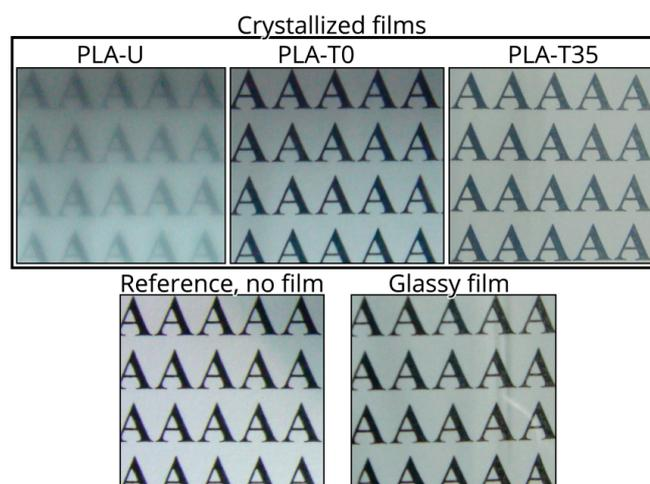
**Figure 9.** See-through (on the top on a text page) macrographs of PLA films of 20  $\mu\text{m}$  thickness, fully crystallized at 110  $^{\circ}\text{C}$ . For comparison, the pictures of reference with no film and glassy one are also shown in lower row.
