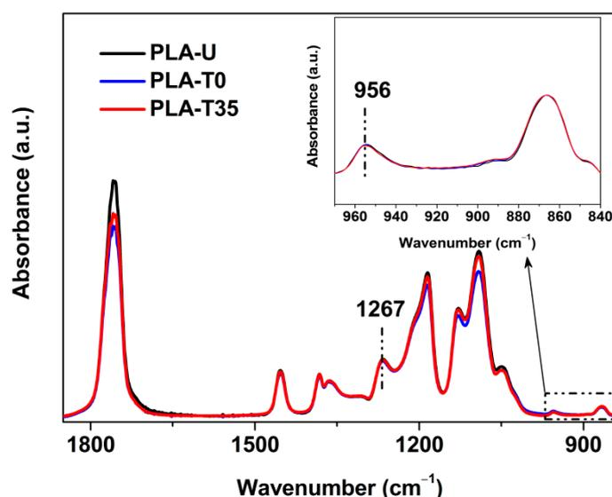
**Figure 10.** FTIR spectra in the 1850–840  $\text{cm}^{-1}$  and 970–840  $\text{cm}^{-1}$  (see the inset) ranges for PLA-U, PLA-T35, and PLA-T0 before further annealing.
