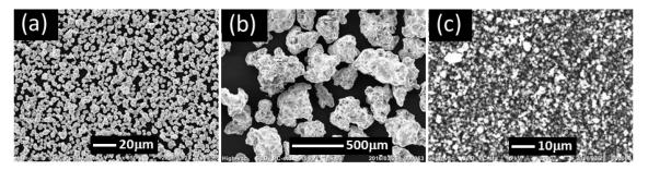
Figure 1. SEM photographs of magnetic and nonmagnetic particles. (a) SP, (b) LP, and (c) NP.
