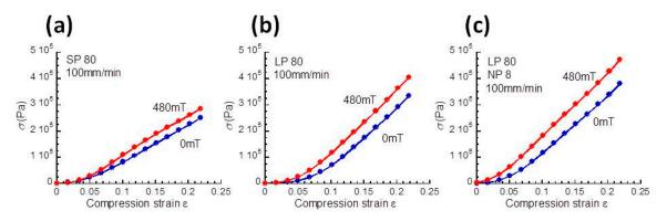
**Figure 3.** Strain–stress curves at 0 and 480 mT for magnetic elastomers containing (**a**) SP, (**b**) LP, and (**c**) LP+NP.
