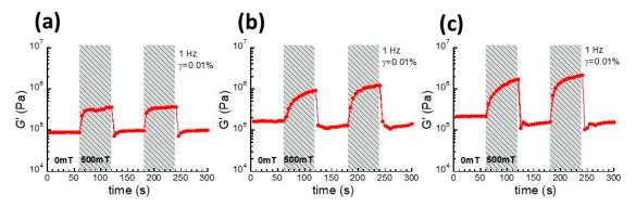
**Figure 2.** Magnetic field responses of the storage modulus under the linear viscoelastic regime for magnetic elastomers containing (**a**) SP, (**b**) LP, and (**c**) LP+NP.
