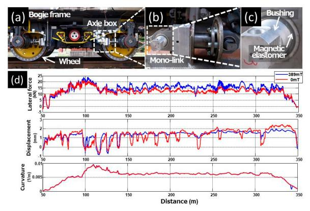
**Figure 4.** Photographs of (**a**) bogie and (**b**,**c**) mono-link made of magnetic elastomer containing LP+NP, (**d**) lateral force (**top**), displacement of the magnetic elastomer bushing (**middle**), and curvature (**bottom**) as a function of running distance.
