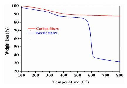
Figure 5. Thermal stability of the carbon fibers and Kevlar fibers.
