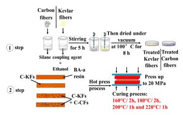
Figure 1. Preparation steps used for the elaboration of the hybrid composites.
