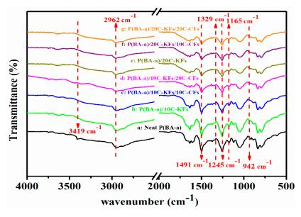
Figure 3. FTIR of the hybrid composites with different hybrid fiber contents.
