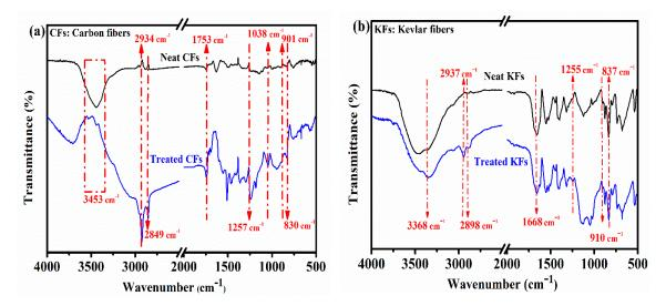
Figure 2. FTIR spectra of the treated and untreated carbon fibers (a) and Kevlar fibers (b).
