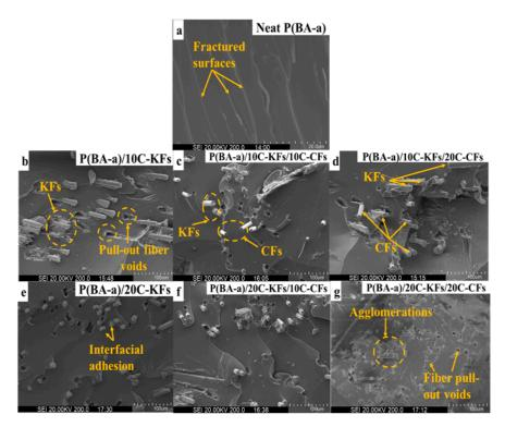
Figure 9. SEM micrographs of the hybrid benzoxazine composites.
