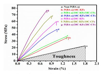
Figure 7. Tensile stress/strain curves of the P(BA-a)/C-KFs/C-CFs composites.
