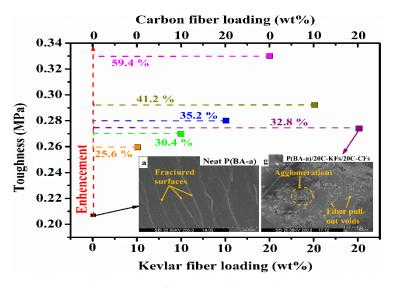
Figure 8. Toughness curve of the P(BA-a)/C–KFs/C–CFs composites.
