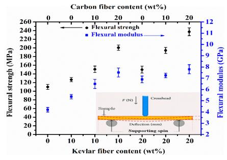
Figure 6. Bending properties of the hybrid benzoxazine composites.
