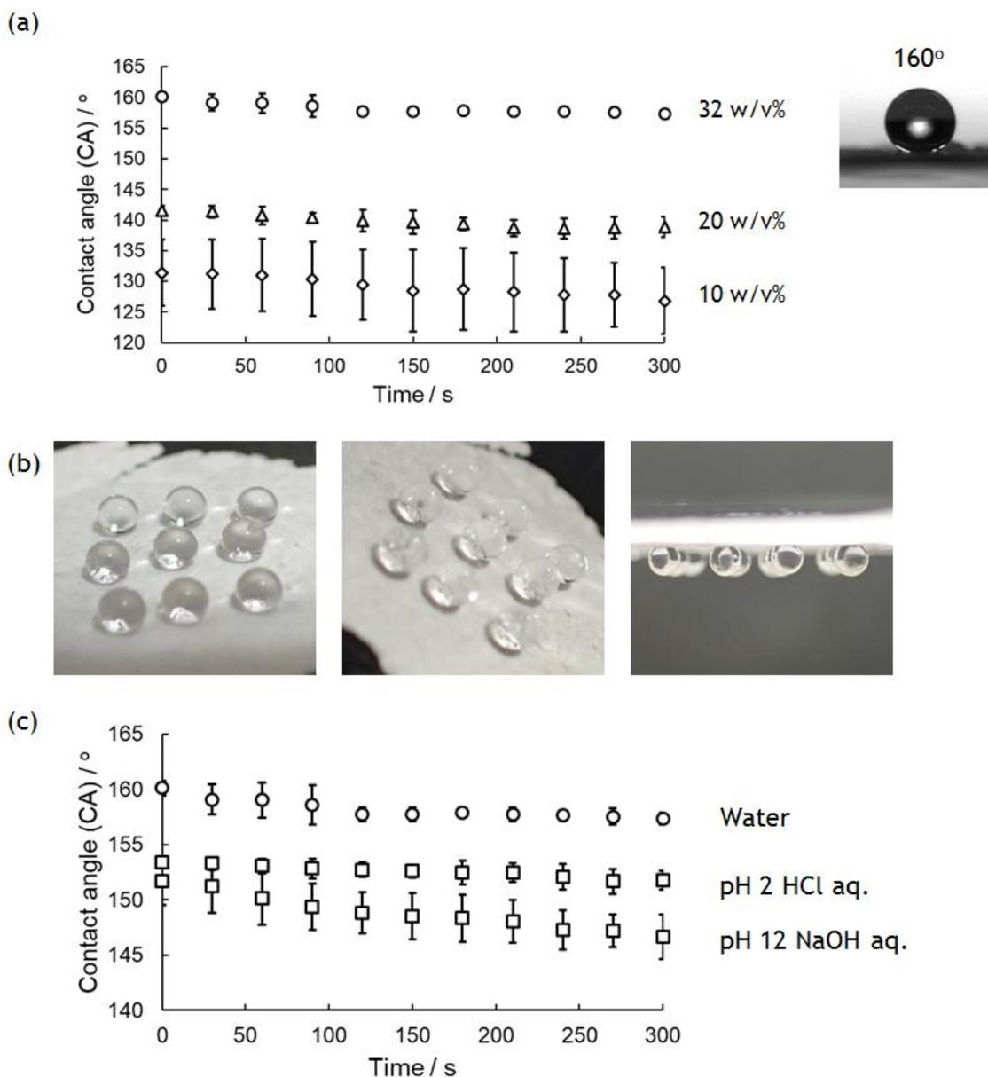
**Figure 4.** Wettability of PolyPhe nonwovens prepared by electrospinning into hexane/ $\text{CHCl}_3$  (9/1  $v/v$ ). (a) CA change on PolyPhe nonwovens electrospun at different polymer concentrations ( $n = 3$ ). (b) Strong adhesion of water droplet onto PolyPhe nonwovens with a tilt angle of 0, 45, and  $90^\circ$ . (c) CA change of acidic (pH 2) and basic (pH 12) droplets on the nonwovens (32  $w/v\%$ ) ( $n = 3$ ).
