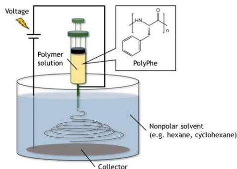
**Figure 1.** The experimental setup for electrospinning used in this study. All processes including spinning were done in a nonpolar solvent.
