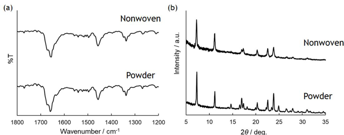
**Figure 3.** (a) FT-IR spectra and (b) XRD patterns of as-synthesized and nonwoven PolyPhe prepared by electrospinning of 32 *w/v*% solution.
