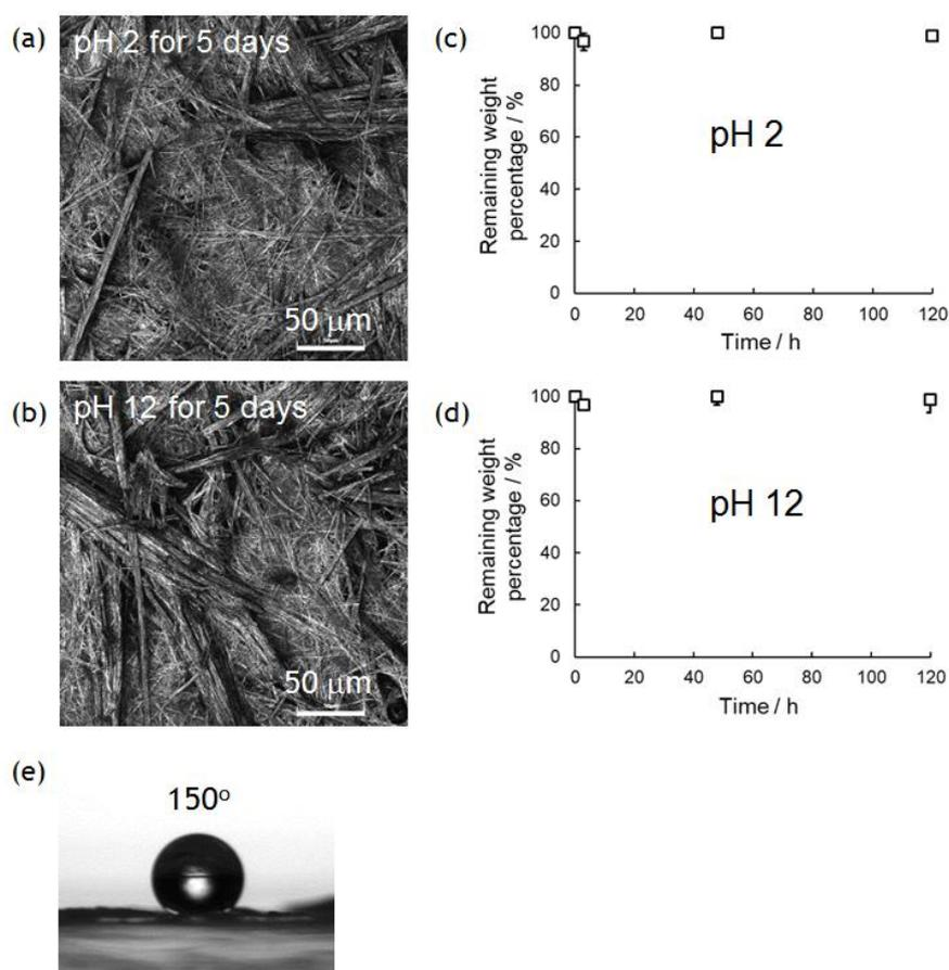
**Figure 5.** Chemical stability of PolyPhe nonwovens prepared by electrospinning into hexane/ $\text{CHCl}_3$  (9/1 *v/v*) in acidic (pH 2) and basic (pH 12) conditions. (a,b) Weight remaining ( $n = 3$ ) and (c,d) LM images of the PolyPhe nonwovens after 5 days' immersion in (a,c) 0.01 M HCl aq. and (b,d) 0.01 M NaOH aq. (e) The CA of a water droplet on the PolyPhe nonwovens after the alkali treatment.
