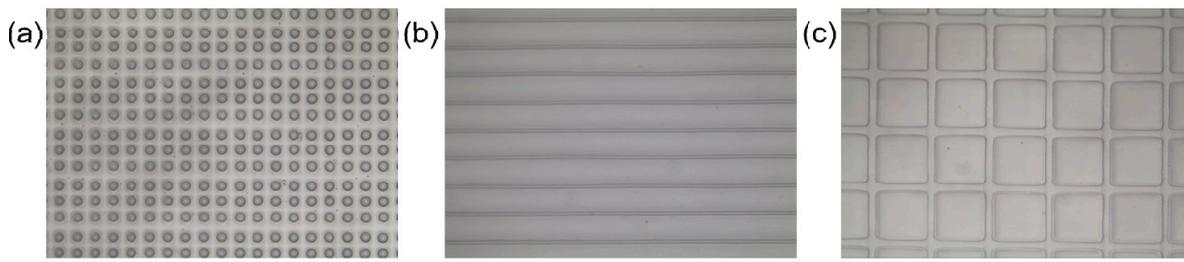
**Figure 3.** Morphologies of fabricated microstructured surfaces based on the etched template. (a) The microstructured surface with raised dot. (b) The microstructured surface with raised line. (c) The microstructured surface with raised square. Scale bar: 200  $\mu\text{m}$ .
