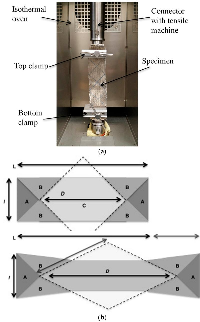
**Figure 3.** (a) Bias extension test set up of the tensile machine with the specimen and (b) Undeformed rectangular specimen and deformed shape of the specimen showing half shear and full shear zone.
