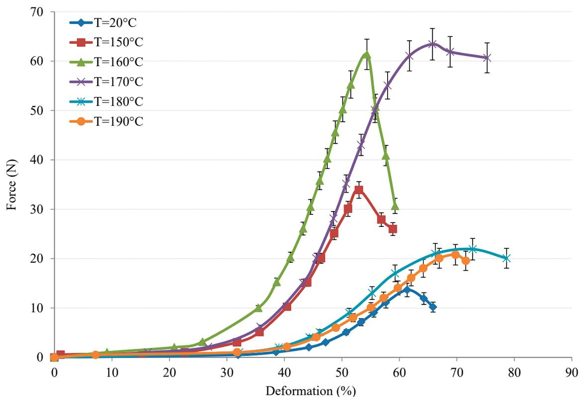
**Figure 8.** The load vs. deformation under variation of temperature.
