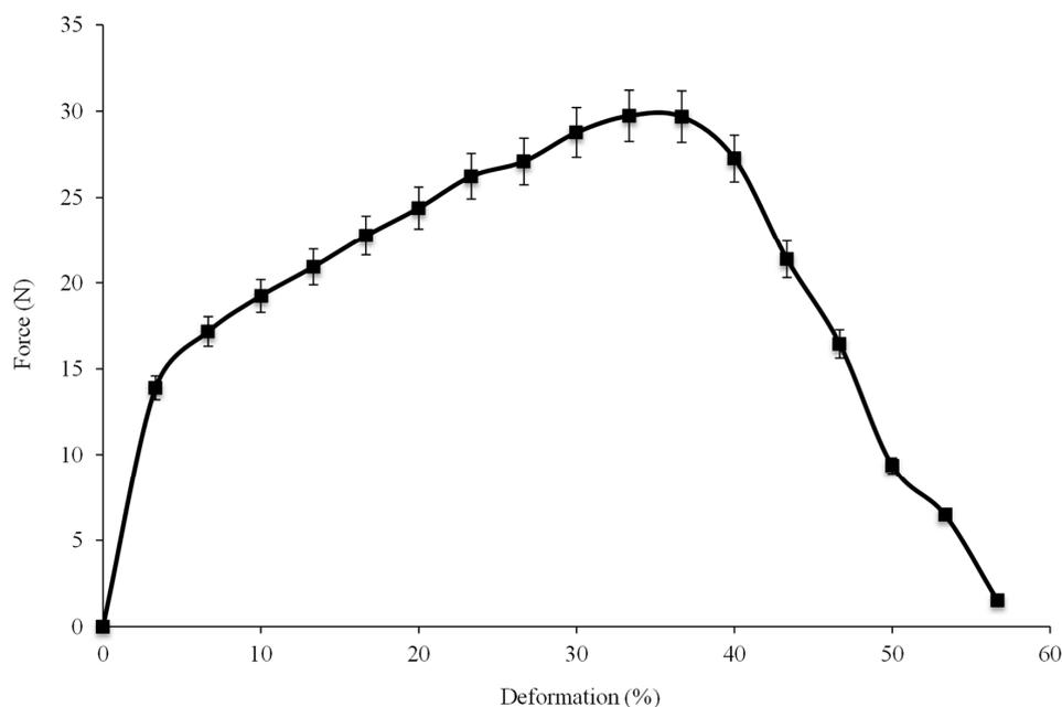
**Figure 4.** Tensile result of single flax/PA12 yarn.
