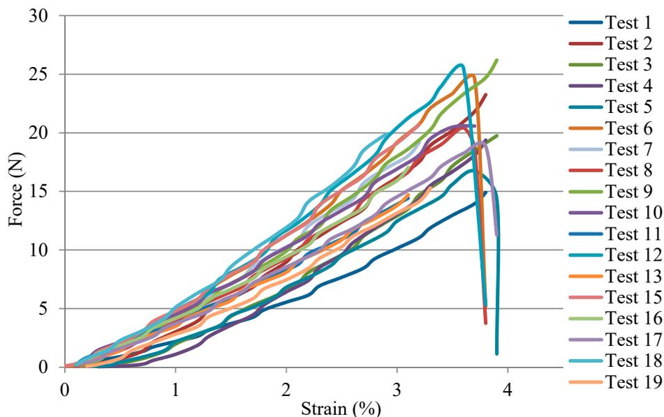
Figure 5. Tensile results of pure flax yarns [28].
