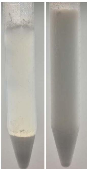
**Figure 6.** Powders *i* (left) and *d* (right) redispersed after spray drying.
