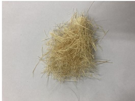
**Figure 1.** Photograph of the short sisal fiber.**Table 3.** Physical and mechanical properties of the sisal fiber (from Hejazi et al. 2012 [1]).
