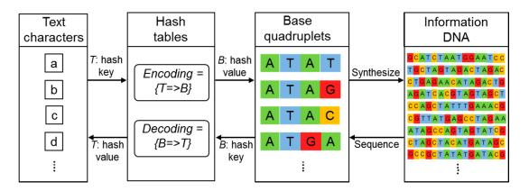
**Figure 1.** Processes of encoding and decoding. These processes were implemented in a Perl script. The schematic thus contains some Perl-style pseudo-codes. See Materials and Methods for details.
